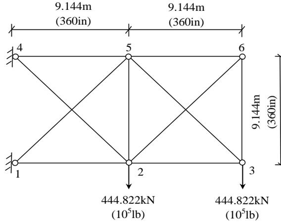
Fig. 9 10-bar truss structure
