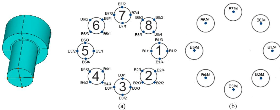
Fig. 4 Nomenclature of selected nodes on bolt shank (a) side nodes (b) mid nodes
