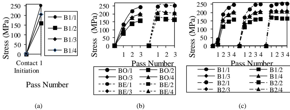
Fig. 7 Bolt bending behavior using stretch control method for four bolts: (a) SC100 (b) SC50 (c) SC33. (BO: Odd numbered bolts, BE: Even numbered bolts)
