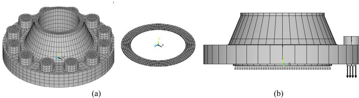
Fig. 1 (a) Meshing of flange and bolt and gasket, (b) applied boundary conditions
