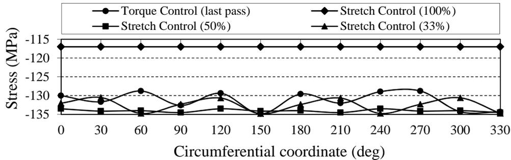
Fig. 8 Gasket stress variation using both methods
