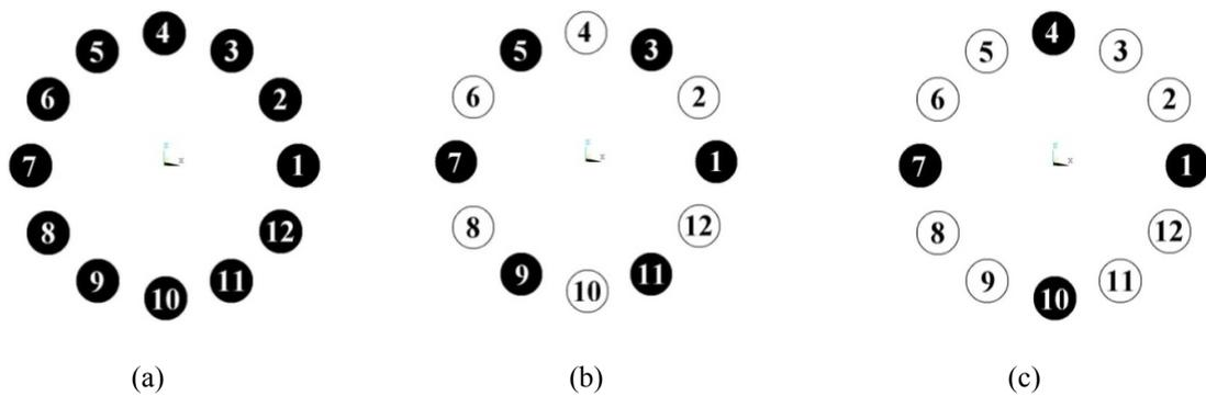
Fig. 3 Percentage of bolts stretched at a time (a) 100% (b) 50% (c) 33%
