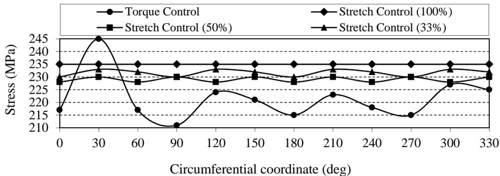
Fig. 9 Principal axial stress variation at hub flange fillet using both methods
