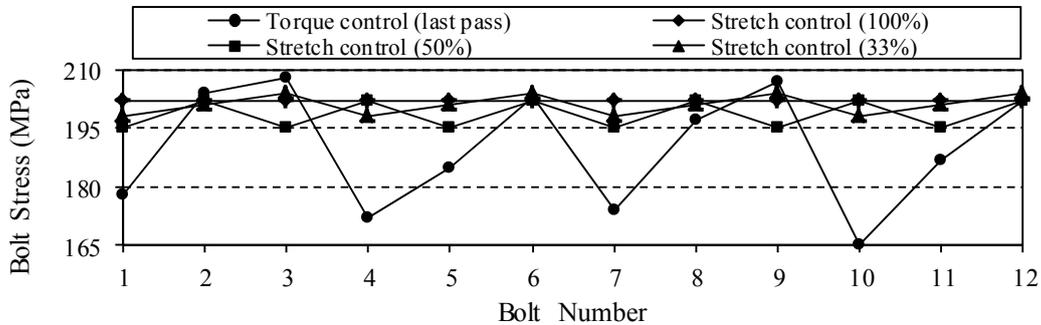
Fig. 5 Axial bolt stress variation using torque control and stretch control methods
