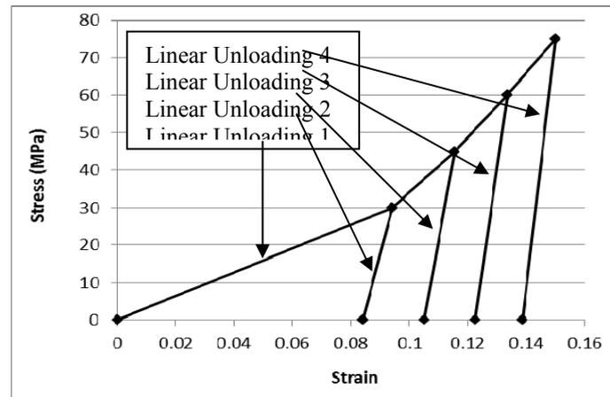
Fig. 2 Loading and unloading curves for the gasket material
