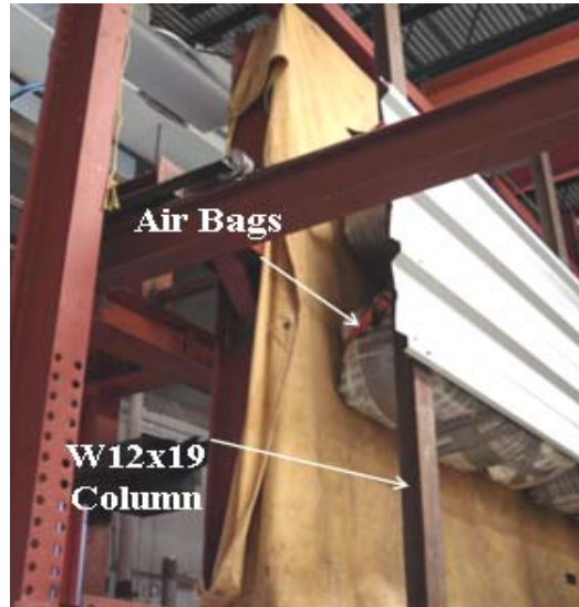
Fig. 2 Side view of test specimen, showing air bags. Panel Type E, gage 24
