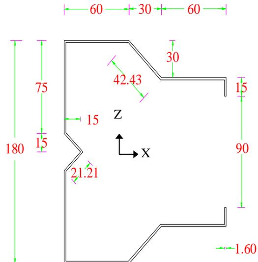
Fig. 3(b) Type-II (Channel) columns
