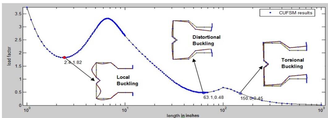
Fig. 2 Typical buckling plot for Type-I (Hat) section columns
