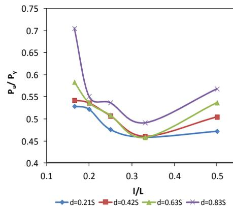
Fig. 13  $P_u/P_y$  Vs  $I/L$  for T2-C series
