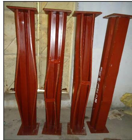
Fig. 5(b) Deformed shape of Type-II columns
