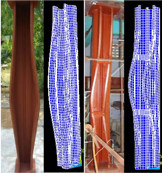
Fig. 8 Correlation of FEA with test results
