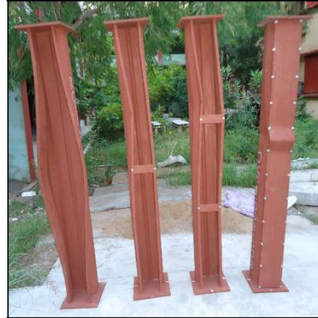
Fig. 5(a) Deformed shape of Type-I columns
