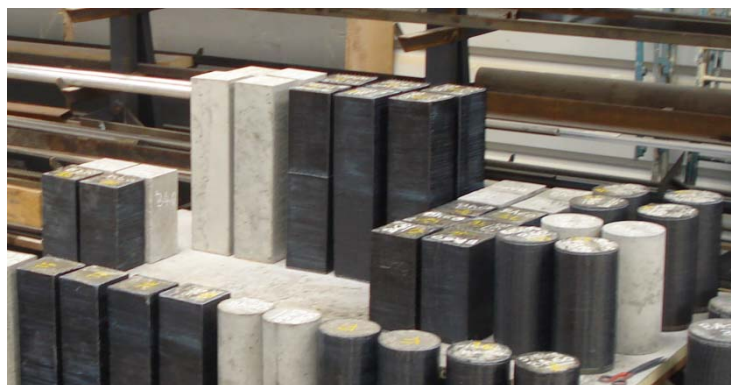
Fig. 3 Samples of specimens after curing and wrapping
