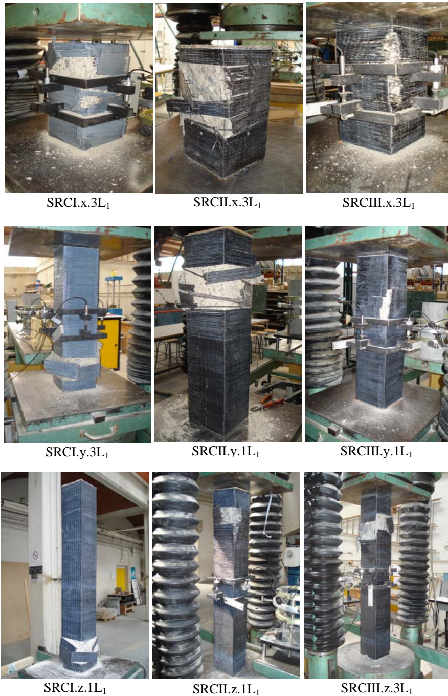
Fig. 5 Typical failure modes for the tested CFRP-confined columns
