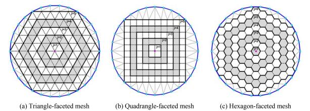
Fig. 3 Schematic of the cyclosymmetry method
