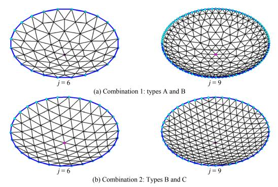
Fig. 7 Spatial mesh configurations by using the topological mapping method (Perspective view)
