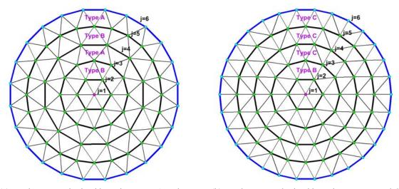
(a) Mesh pattern obtained by using types A and B
