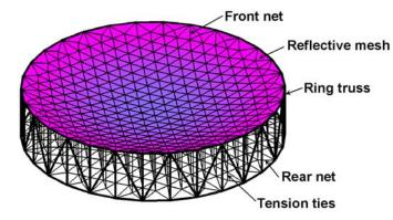
Fig. 1 Structural construction of a typical cable-network antenna reflector
