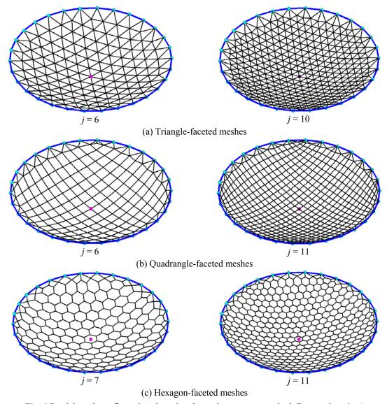
Fig. 6 Spatial mesh configurations by using the cyclosymmetry method (Perspective view)
