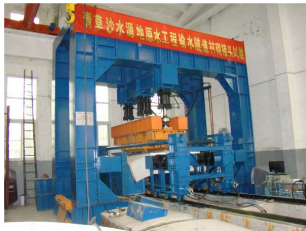
Fig. 3 Newly developed testing facility for full-scale joint tests
