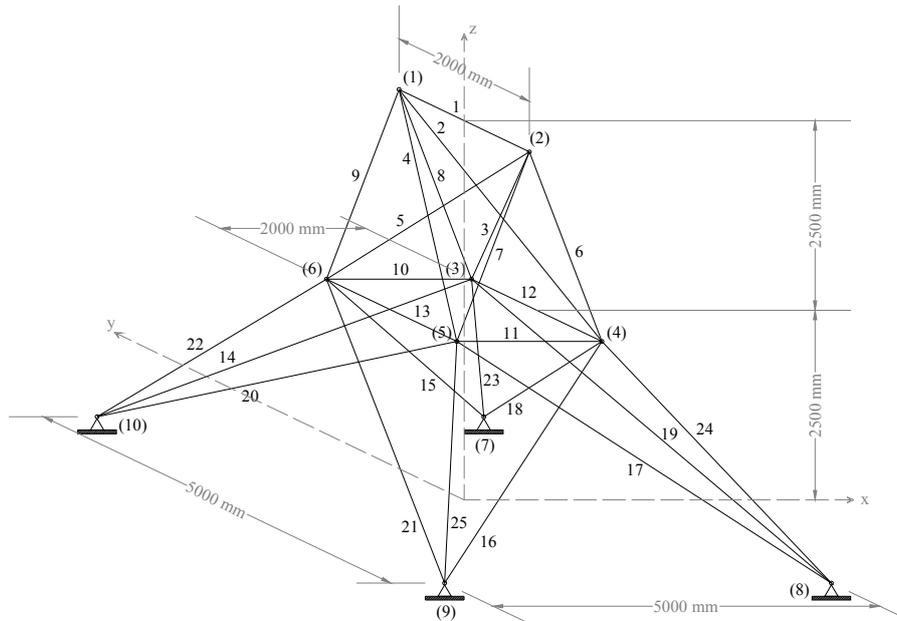
Fig. 7 25-bar space truss
