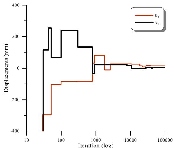
Fig. 5 Variation of displacements  $u_4$  and  $v_5$  in the 6-bar truss with respect to the number of iterations
