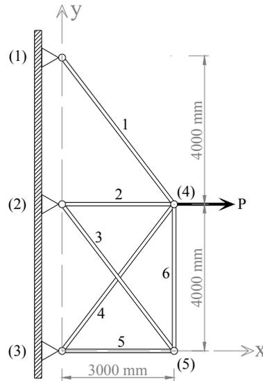
Fig. 3 6-bar plane truss
