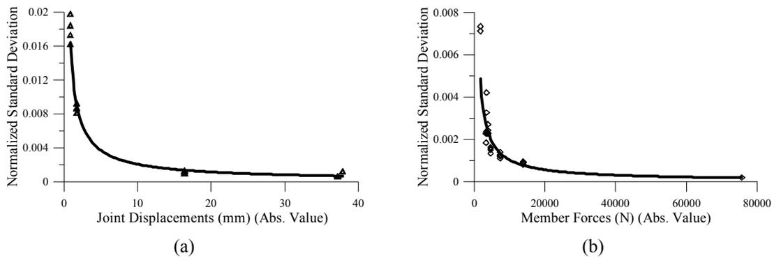
Fig. 9 Normalized standard deviations in 100 independent runs for the 25-bar space truss under Loading 1, solutions with  $p = 20$  vectors (a) Joint displacements (b) Members Forces
