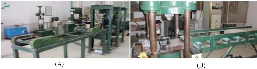
Fig. 1 Cracking facilities (A) central-cracking static-press (B) rail-seat-cracking static-press
