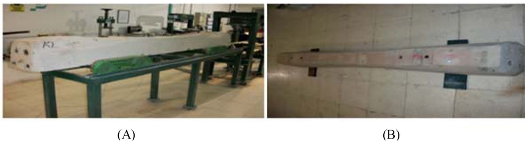
Fig. 3 (A) Support system for central cracked sleeper testing (B) support system for rail seat cracked sleeper testing
