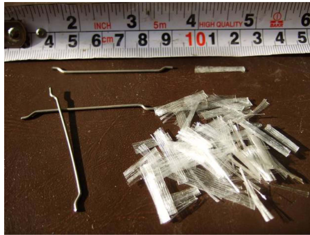
Fig. 2 Steel and polypropylene fibers
