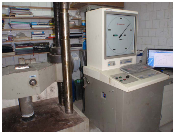
Fig. 3 Compression test of concrete cylinders
