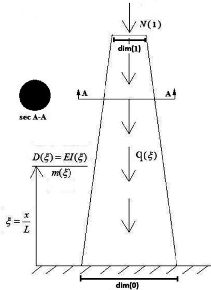
Fig. 3 The non-prismatic cantilever beam with circular cross section under variable axial forces
