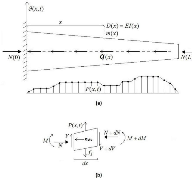
Fig. 1 (a) Bernoulli beam vibration under variable axial forces and transverse forces, (b) resultant forces acting on a differential element
