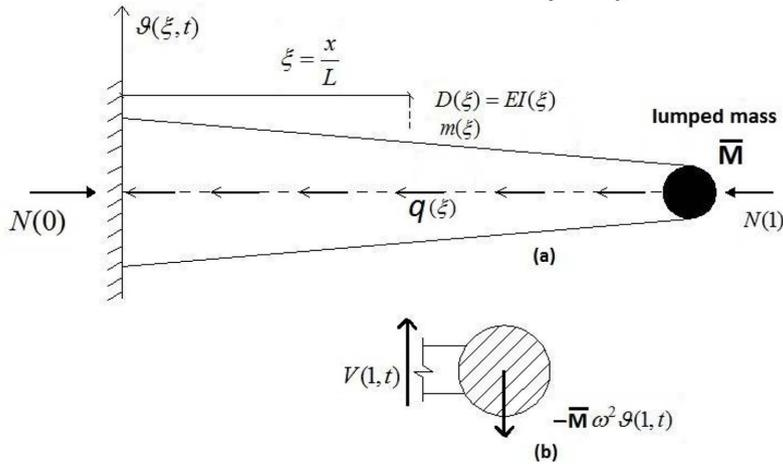
Fig. 2 (a) cantilever beam vibration with a lumped mass at free end, (b) shear force acting on the end mass
