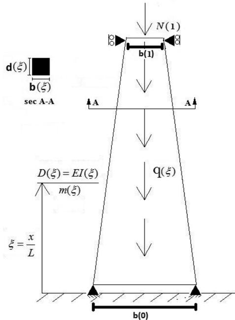
Fig. 5 The non-prismatic simply supported beam with square cross section, under variable axial forces
