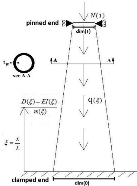
Fig. 4 The non-prismatic clamped-pinned beam with hollow circular cross section, under variable axial forces
