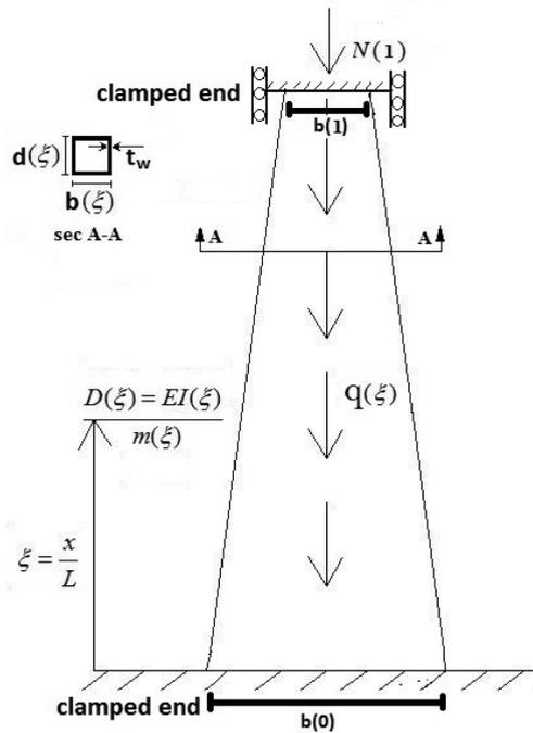
Fig. 6 The non-prismatic clamped-clamped beam with hollow square cross section, under variable axial force
