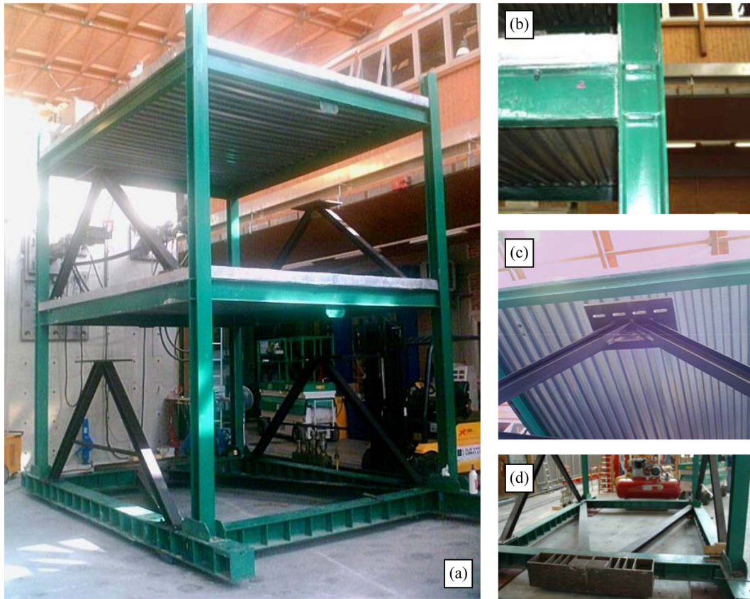
Fig. 1 The structural prototype: (a) overall view, (b) beam-column joint, (c) gusset plates atop V-inverted braces, (d) rigid steel base
