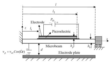
Fig. 1 The configuration of system under combined electrostatic and piezoelectric actuations
