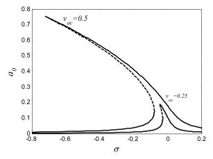
Fig. 13 Variations of  $a_0$  with respect to the variations of  $\sigma$  for different values of  $v_{ac}$  where  $\alpha_2 v_p^2 = 60$ . Solid lines belong to stable solution, and dashed lines belong to unstable solution
