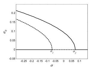
Fig. 6 Variations of  $a_0$  with respect to the variations of  $\sigma$  for the system with  $\alpha_2 v_p^2 = 55$ ,  $v_{ac} =$ 0.06, S < 0 Solid lines belong to stable solution, and dashed lines belong to unstable solution
