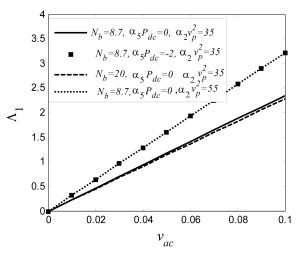
Fig. 3 Variations of  $\Lambda_1$  with respect to the variations of  $v_{ac}$  for different values of system parameters, where,  $\alpha_2 = 2.95$ ,  $h_p/h_b = 0.1$ ,  $v_{ac} = 0.02$ ,  $\mu = 0.04$ ,  $l_2 - l_1 = 0.4l$
