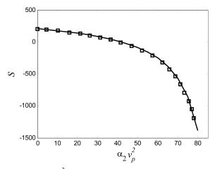
Fig. 2 Variations of S with respect to  $\alpha_2 v_p^2$  for a microbeam without piezoelectric layer, N = 8.7, and  $a_b = 3.7$ ; the square points belong to Younis and Nayfeh (2003), the solid lines belong to Zamanian and Khadem (2010)
