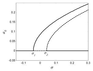
Fig. 5 Variations of  $a_0$  with respect to the variations of  $\sigma$  for system with  $\alpha_2 v_p^2 = 35$ ,  $v_{ac} = 0.06$ , S > 0. Solid lines belong to stable solution, and dashed lines belong to unstable solution
