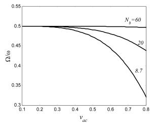
Fig. 9 The effect of  $v_{ac}$  and  $\alpha_2 v_p^2$  on the nonlinear shift of resonance frequency
