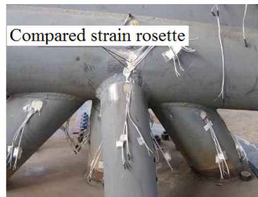
Fig.7 Compared strain rosette on specimen
