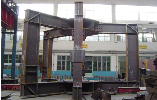
Fig. 3 Self-balance loading frame
