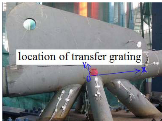
Fig. 6 Location of transfer grating on specimen
