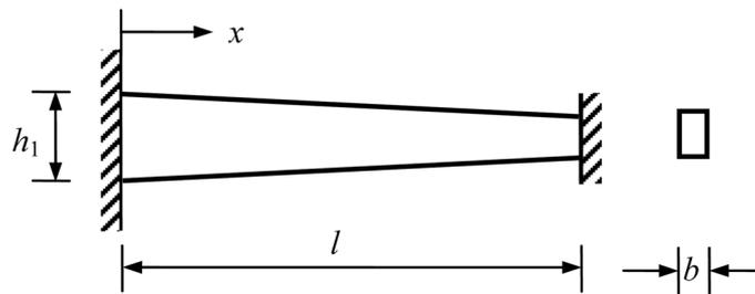
Fig 6. A clamped-clamped tapered Timoshenko beam
