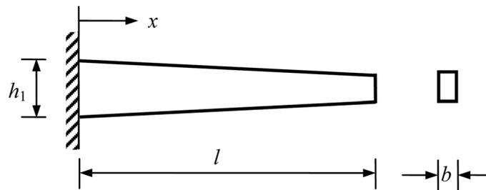
Fig 4. A cantilever tapered Timoshenko beam
