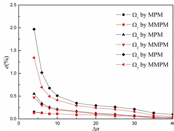
Fig 5. Relative error of the first three frequencies by MPM and MMPM
