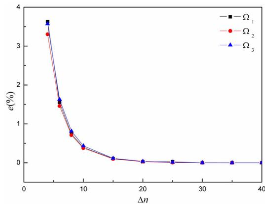
Fig 3. Relative error of first three frequencies:  $E/G = 2.6$ ,  $\chi = 5/6$ ,  $r = 0.0707$  and  $\alpha = -0.9$
