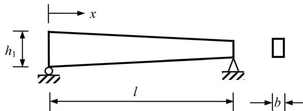
Fig 1. A simply-supported tapered beam
