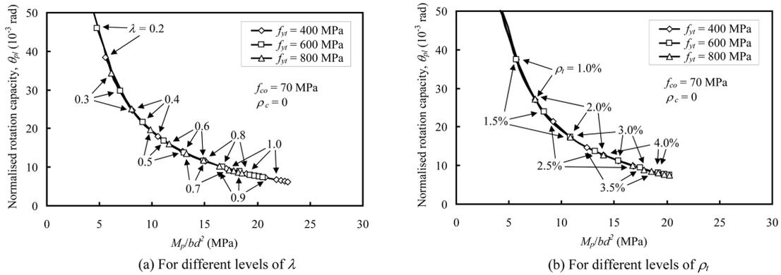
Fig. 4 Maximum limits of flexural strength and deformability for beams with different tension steel yield strength
