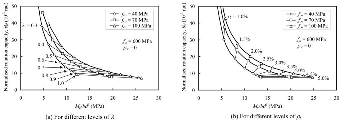
Fig. 3 Maximum limits of flexural strength and deformability for beams with different concrete strength
