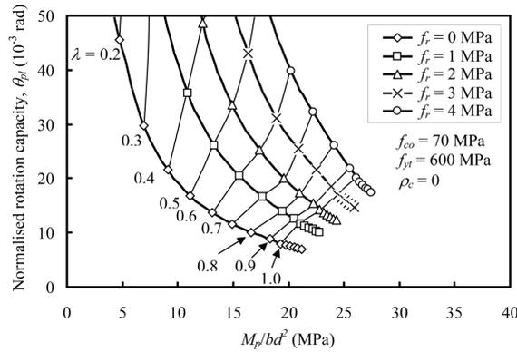
Fig. 8 Maximum limits of flexural strength and deformability for beams with different confining pressure (II)
