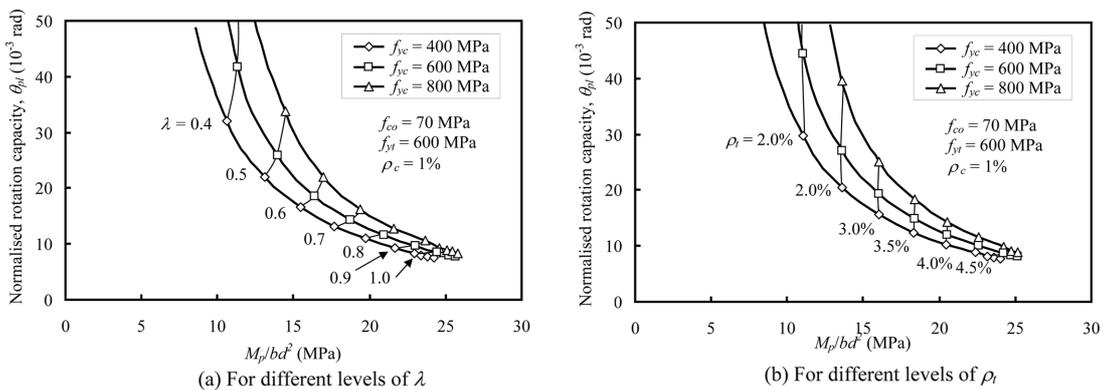
Fig. 6 Maximum limits of flexural strength and deformability for beams with different compression steel yield strength
