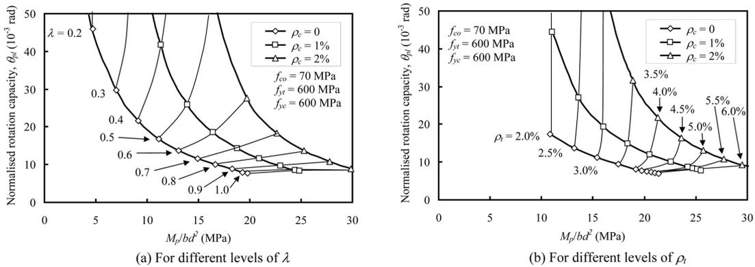
Fig. 5 Maximum limits of flexural strength and deformability for beams with different compression steel ratios
