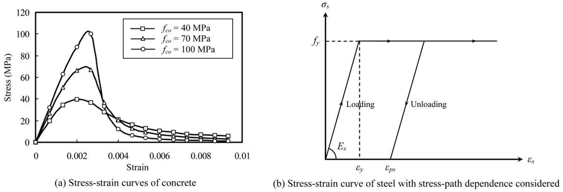
Fig. 1 Stress-strain curves of concrete and steel reinforcement
