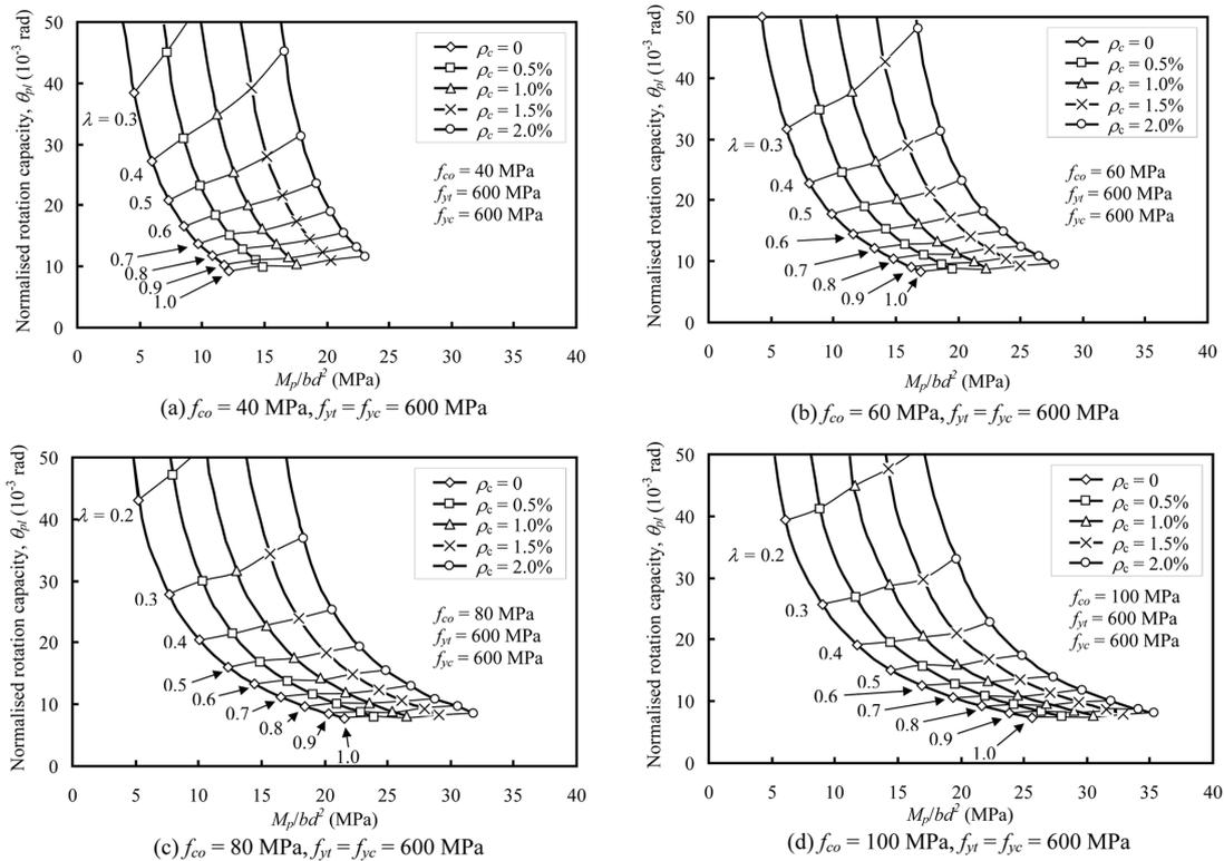
Fig. 10 Design charts for beams with different compression steel ratios
