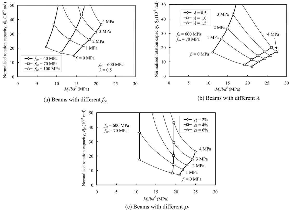
Fig. 7 Maximum limits of flexural strength and deformability for beams with different confining pressure (I)
