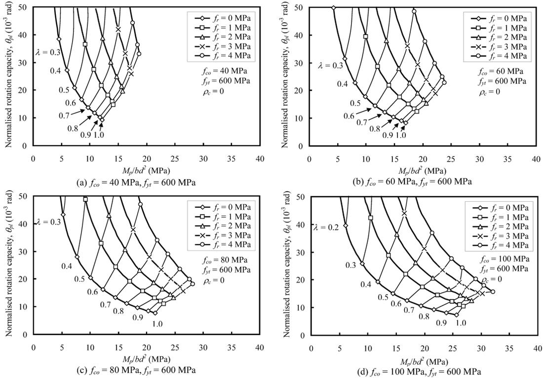
Fig. 11 Design charts for beams with different confining pressure
