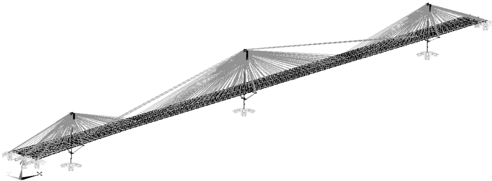
Fig. 2 Full grid beam model of Ting Kau Bridge
