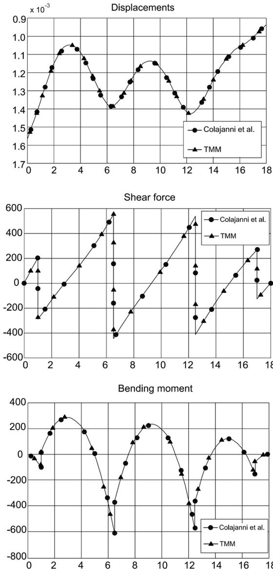
Fig. 4 Displacement [m], Shear force [kN] and bending moment [kNm] diagrams of example 1. Bernoulli beam
