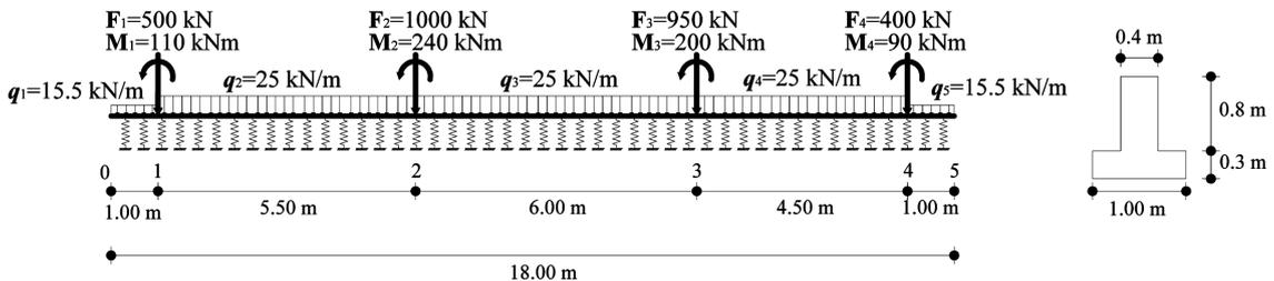
Fig. 3 Geometric characteristics of rectilinear beam of example 1
