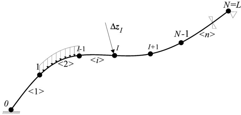
Fig. 2 Complex structure divided into segments with general boundaries and actions applied
