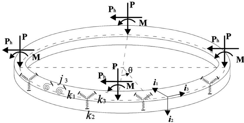
Fig. 7 Loads on the ring for horizontal actions on the tank
