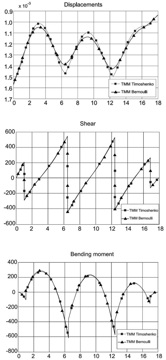
Fig. 5 Comparison between TMM with and without shear stiffness. Displacements [m], shear [kN] and bending moment [kNm] diagrams of example 1
