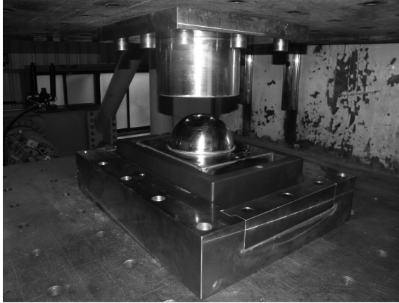
Fig. 13 Specimen of the MTFPS isolator in the X direction for the component test
