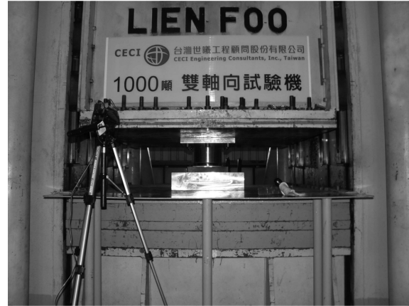
Fig. 14 Test set-up for the component test of the MTFPS isolator
