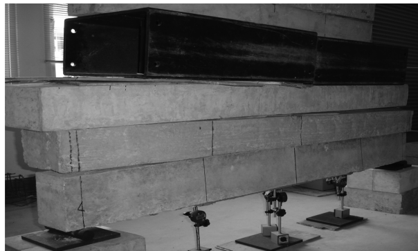
Fig. 6 Long-term deflection test setup
