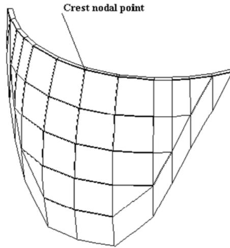
Fig. 3 Finite element mesh of Morrow Point dam (Model B)
