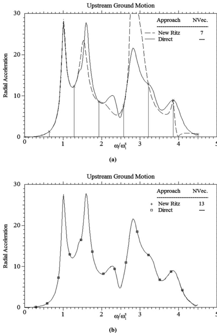
Fig. 6 Response of Model B based on new Ritz method (a) 7 Vectors, (b) 13 Vectors (vertical lines shows the location of new Ritz vectors corresponding frequencies)
