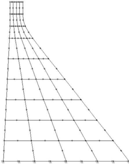
Fig. 2 Finite element discretization of Pine Flat dam (Model A)
