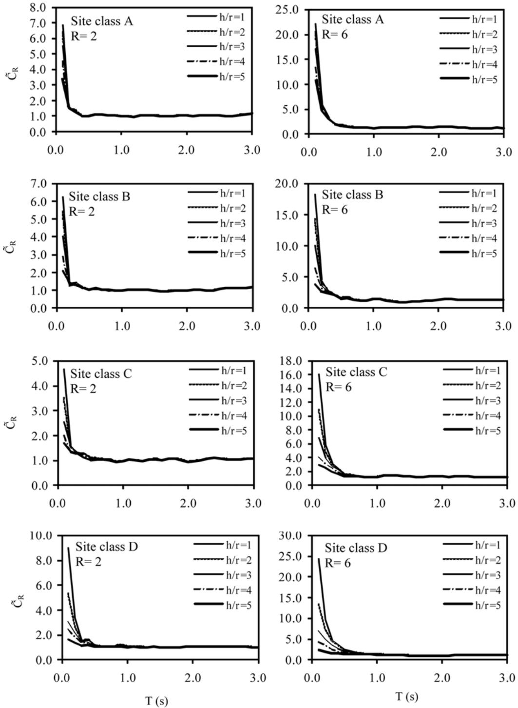
Fig. 6 Variations of mean inelastic displacement ratios against period on different soil types for increasing values of  $h/r$ . Results correspond to an interacting system with  $R = 2$  and 6
