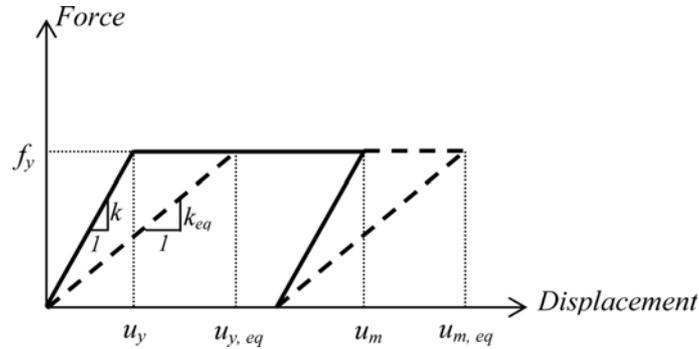
Fig. 3 Force-displacement relationships for the actual structure (solid line) and equivalent fixed-base model (dashed line) (Aviles and Perez-Rocha 2003)
