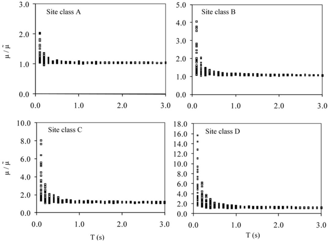
Fig. 10 Ratio of mean ductility demands for cases with and without interaction for all strength reduction levels and aspect ratios
