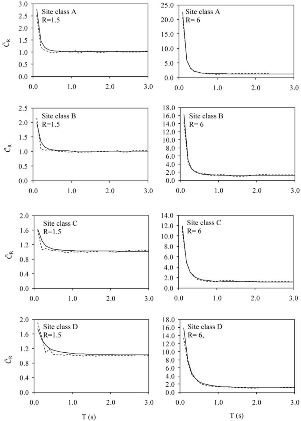
Fig. 11 Comparison of observed (dashed line) and calculated (solid line) mean inelastic displacement ratios (Eq. (11)) of interacting system with  $h/r = 3$  for different soil classes
