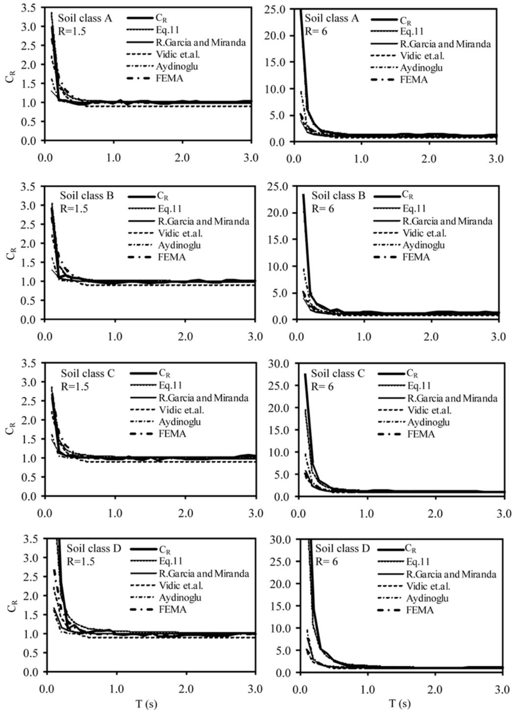
Fig. 12 Comparison of mean inelastic displacement ratios of fixed-base case to those computed with rearranged (Eq. (11)) and other equations in literature
