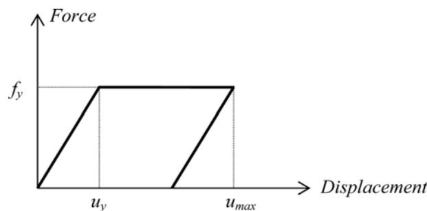
Fig. 1 Elastoplastic model of an SDOF system
