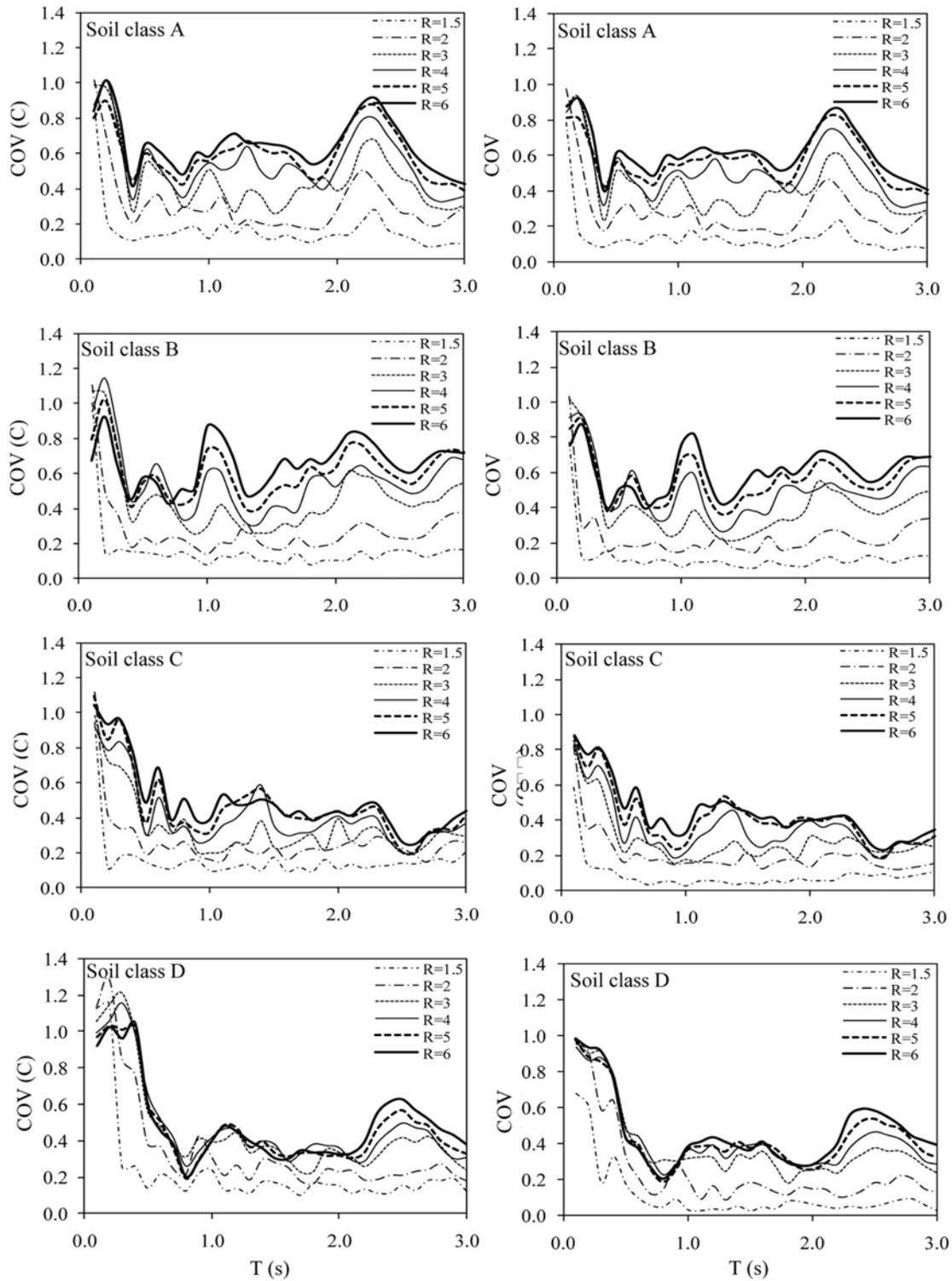
Fig. 4 COVs of inelastic displacement ratios of fixed base and interacting cases
