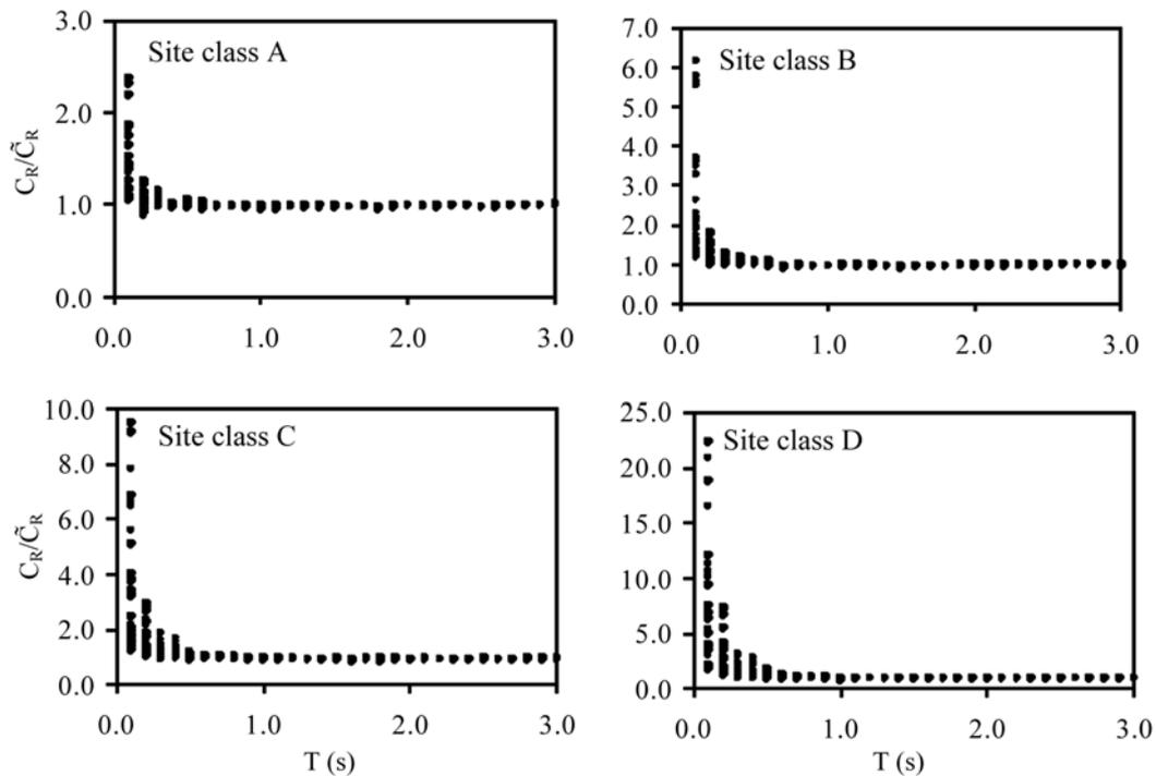
Fig. 7 Ratio of mean inelastic displacement ratios for cases with and without interaction for all strength reduction levels and aspect ratios
