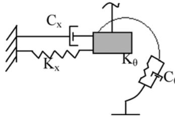
Fig. 2 Mathematical model of support with soil structure interaction
