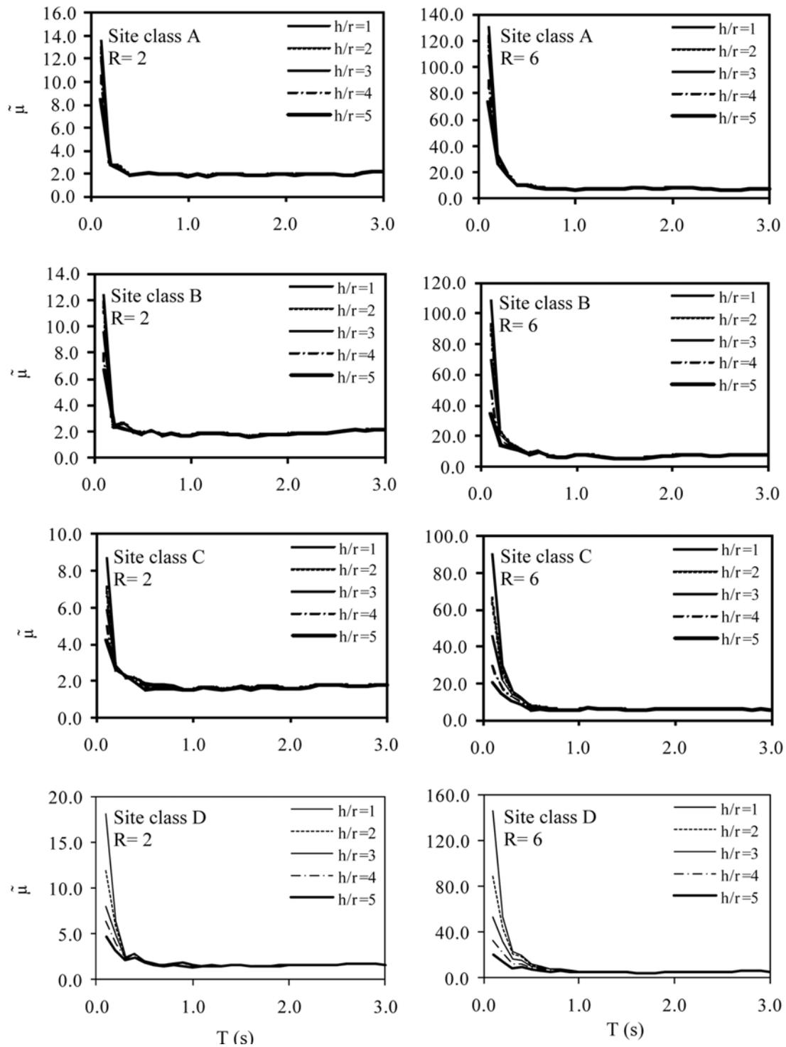
Fig. 9 Variations of mean ductility demands against period on different soil types for increasing values of  $h/r$ . Results correspond to an interacting system with  $R = 2$  and  $6$
