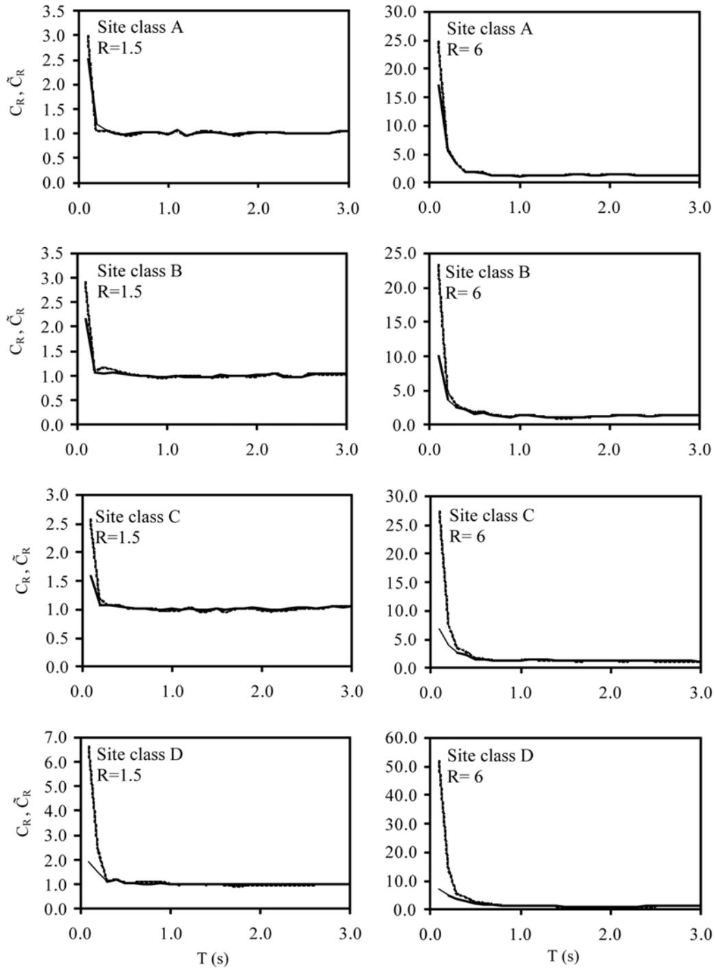
Fig. 5 Variations of mean inelastic displacement ratios against period on different soil types are shown for cases with (solid line) and without (dashed line) interaction for an interacting system with  $R = 1.5$  and 6 and with  $h/r = 3$
