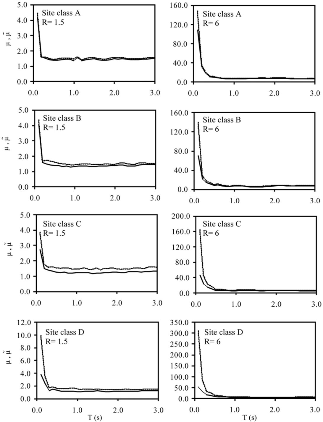
Fig. 8 Variations of mean ductility demands against period on different soil types are shown for cases with (solid line) and without (dashed line) interaction for an interacting system with  $R = 1.5$  and 6 and with  $h/r = 3$
