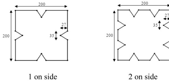
Fig. 10 Cross sections of the concrete-filled steel composite columns (Triangular stiffeners & cold-formed steel sheets of 1.5, 1.75 & 2 mm)
