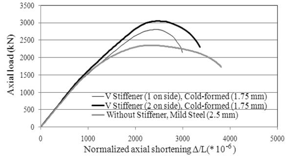
Fig. 16 Axial load-normalized axial shortening plots for columns with different number of V stiffeners (cold-formed 1.75 mm) and without stiffener (mild steel 2.5 mm)
