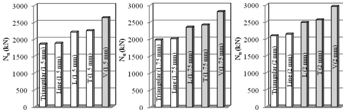
Fig. 26 Effect of shape of steel sheeting stiffeners on ultimate axial load capacity of the columns (1 on side stiffeners)
