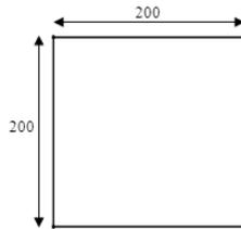
Fig. 1 Cross section of the concrete-filled steel composite column (UCFT2-1, without stiffener, mild steel sheet of 2.5 mm, used by Tao *et al.* 2007) (All dimensions are in mm)
