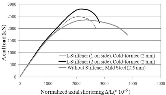
Fig. 23 Axial load-normalized axial shortening plots for columns with different number of L stiffeners (cold-formed 2 mm) and without stiffener (mild steel 2.5 mm)
