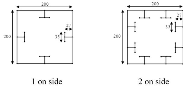
Fig. 7 Cross sections of the concrete-filled steel composite columns (T stiffeners & cold-formed steel sheets of 1.5, 1.75 & 2 mm)
