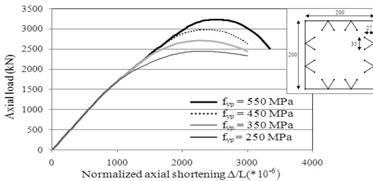
Fig. 32 Effect of yield stress  $f_{yp}$  of cold-formed steel sheet
