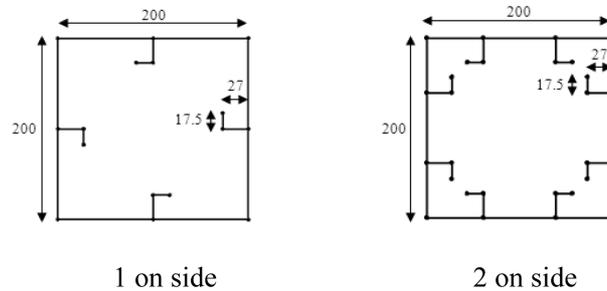
Fig. 8 Cross sections of the concrete-filled steel composite columns (L stiffeners & cold-formed steel sheets of 1.5, 1.75 & 2 mm)
