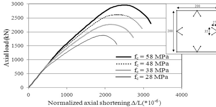
Fig. 29 Effect of concrete compressive strength  $f_c$
