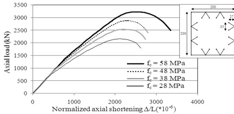
Fig. 30 Effect of concrete compressive strength  $f_c$
