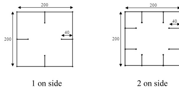
Fig. 9 Cross sections of the concrete-filled steel composite columns (Line stiffeners & cold-formed steel sheets of 1.5, 1.75 & 2 mm)
