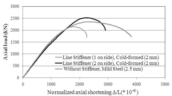
Fig. 24 Axial load-normalized axial shortening plots for columns with different number of Line stiffeners (cold-formed 2 mm) and without stiffener (mild steel 2.5 mm)
