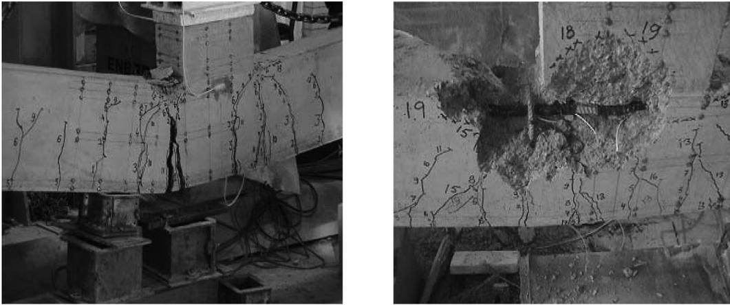
Fig. 2 Extent of crushing at ultimate and buckling of compression steel after failure
