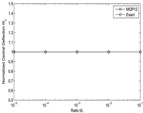
Fig. 16 Normalized central deflections for various thickness-span ratios ( $t/L = 0.00001, 0.0001, 0.001, 0.01$  and  $0.1$ )
