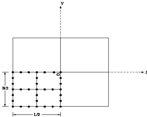
b. A typical  $(2 \times 2)$  mesh in one quadrant of the plate
