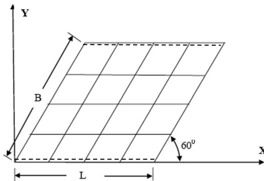
Fig. 4 Razzaque's plate:  $L = 100$ ,  $B = 100$ ,  $t = 1$ ,  $E = 1092000.0$ ,  $\nu = 0.3$  and  $q = 1$ , inclination of the plate  $\theta = 60^\circ$  (Two opposite edges simply supported while other two free)
