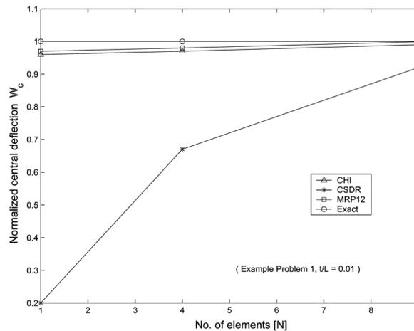
Fig. 10 Normalized central deflection for a clamped square thin plate with central point load
