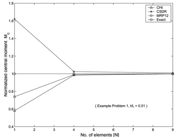
Fig. 7 Normalized central moment for a simply supported square thin plate with uniform load
