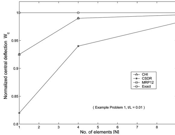
Fig. 9 Normalized central deflection for a simply supported square thin plate with point load
