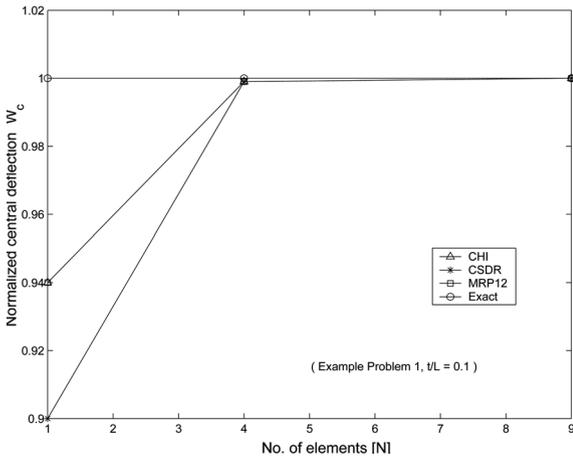
Fig. 11 Normalized central deflection for a simply supported moderately thick square thin plate with uniform load
