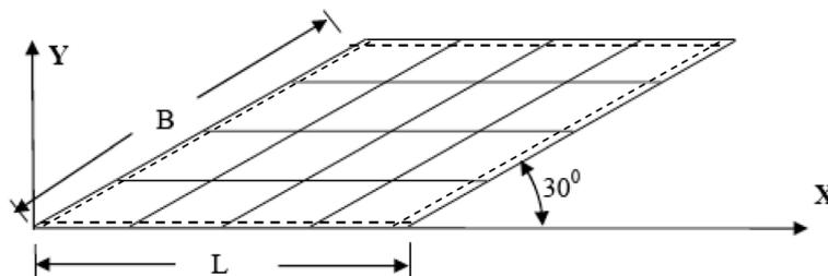
Fig. 3 Morley's plate:  $L = 100$ ,  $B = 100$ ,  $t = 1$ ,  $E = 1092000.0$ ,  $\nu = 0.3$  and  $q = 1$ , inclination of the plate  $\theta = 30^\circ$ ,  $w = 0$  on all sides of the plate
