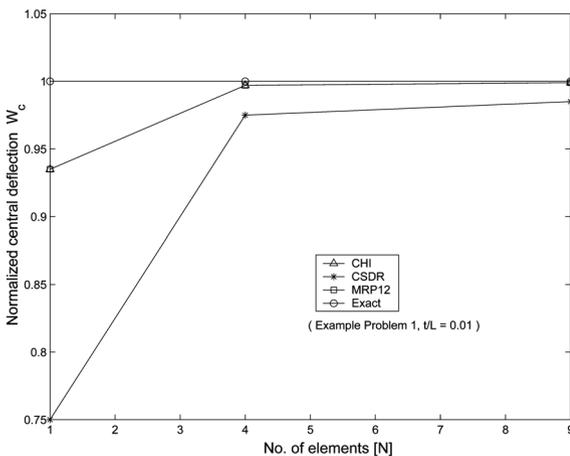
Fig. 6 Normalized central deflection for a simply supported square thin plate with uniform load
