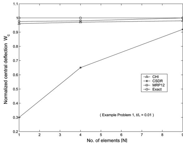
Fig. 8 Normalized central deflection for a clamped square thin plate with uniform load
