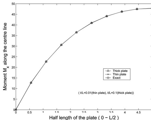
Fig. 13 Variation of moment  $M_x$  along central line of the simply supported square thin/moderately thick plate with uniform load for grid size  $(3 \times 3)$
