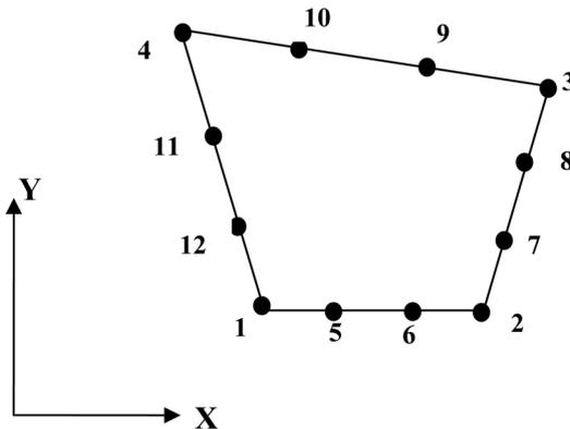
Fig. 1 A typical 12-node quadrilateral plate bending element
