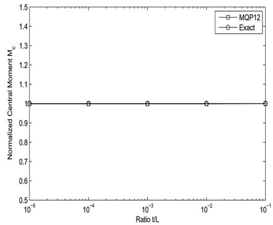
Fig. 17 Normalized central moments for various thickness-span ratios ( $t/L = 0.00001, 0.0001, 0.001, 0.01$  and  $0.1$ )
