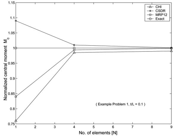
Fig. 12 Normalized central moment for a simply supported moderately thick square plate with uniform load
