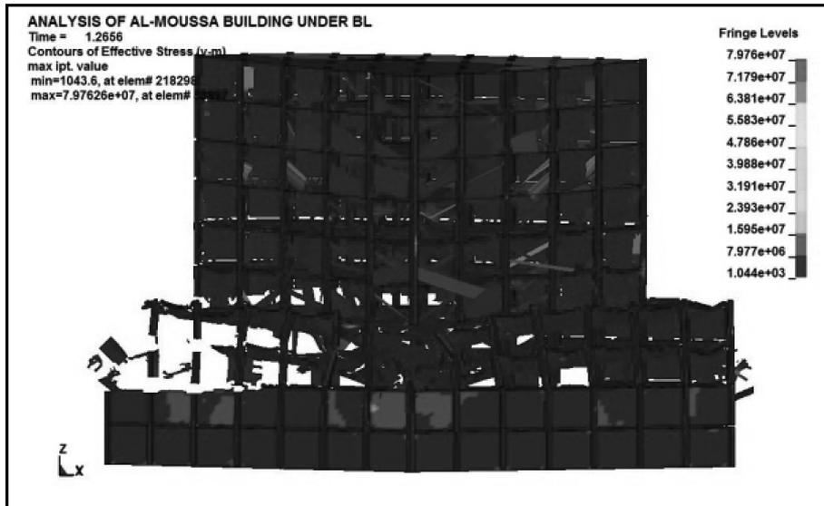
Fig. 9 Damage caused to the entire structure for Scenario 4
