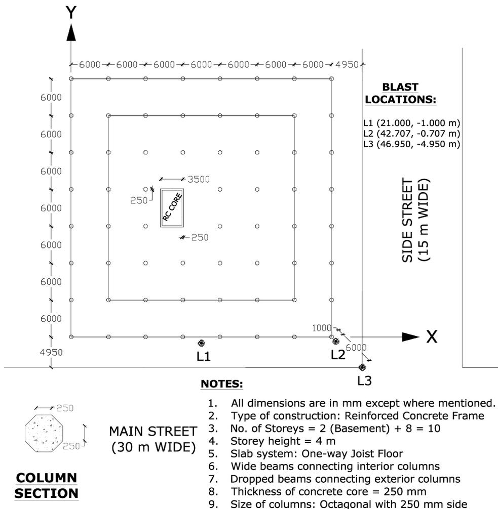
Fig. 5 Location of blast charge for different scenarios
