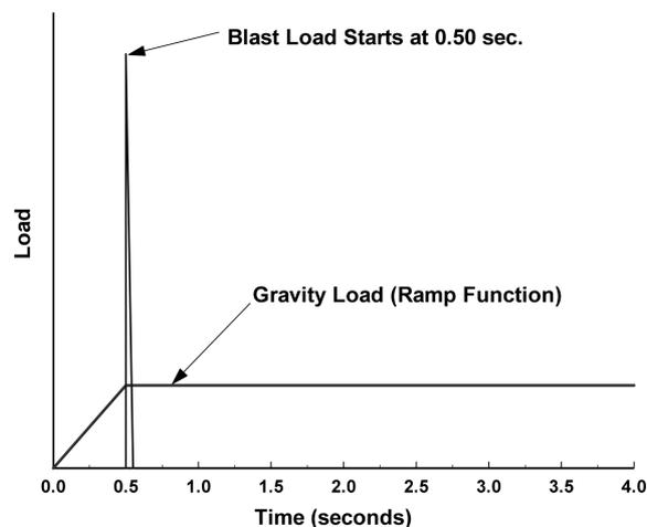
Fig. 4 Loading application for gravity and blast loads
