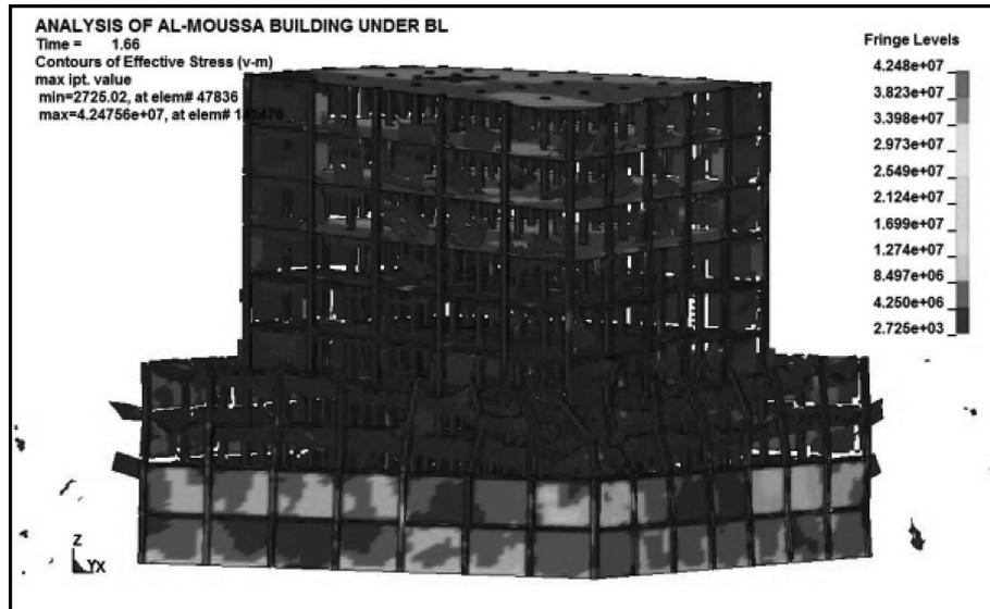
Fig. 7 Damage caused to the entire structure at 1.66 seconds for Scenario 2
