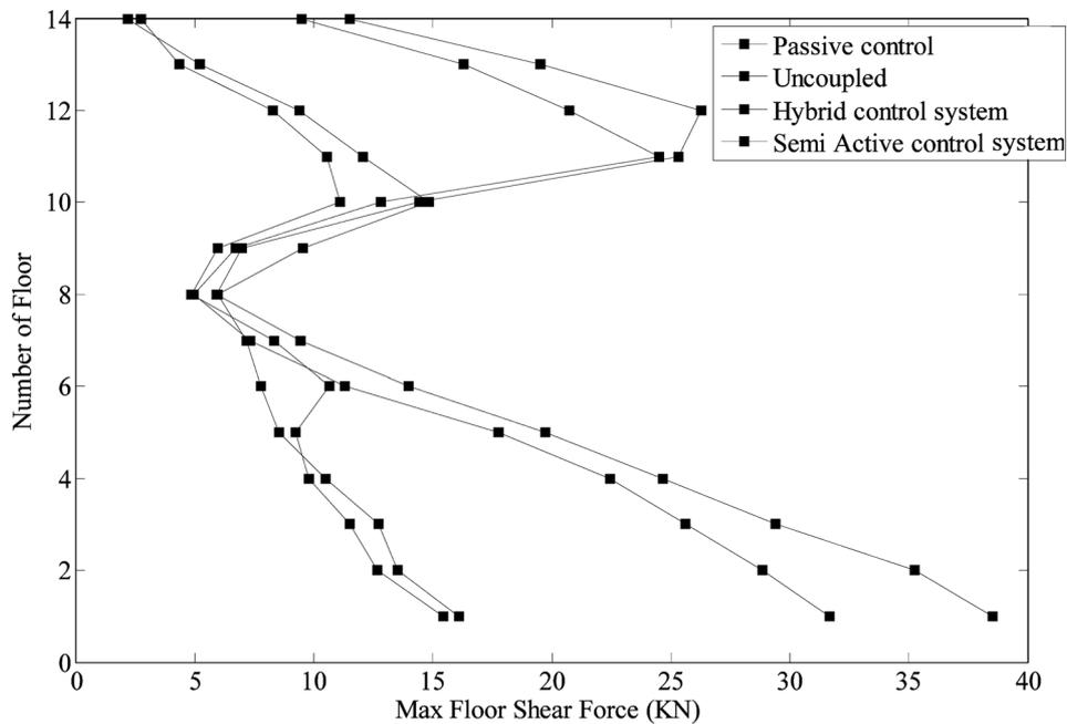
Fig. 6 Maximum shear force in different stories of building 1 in different coupling configurations
