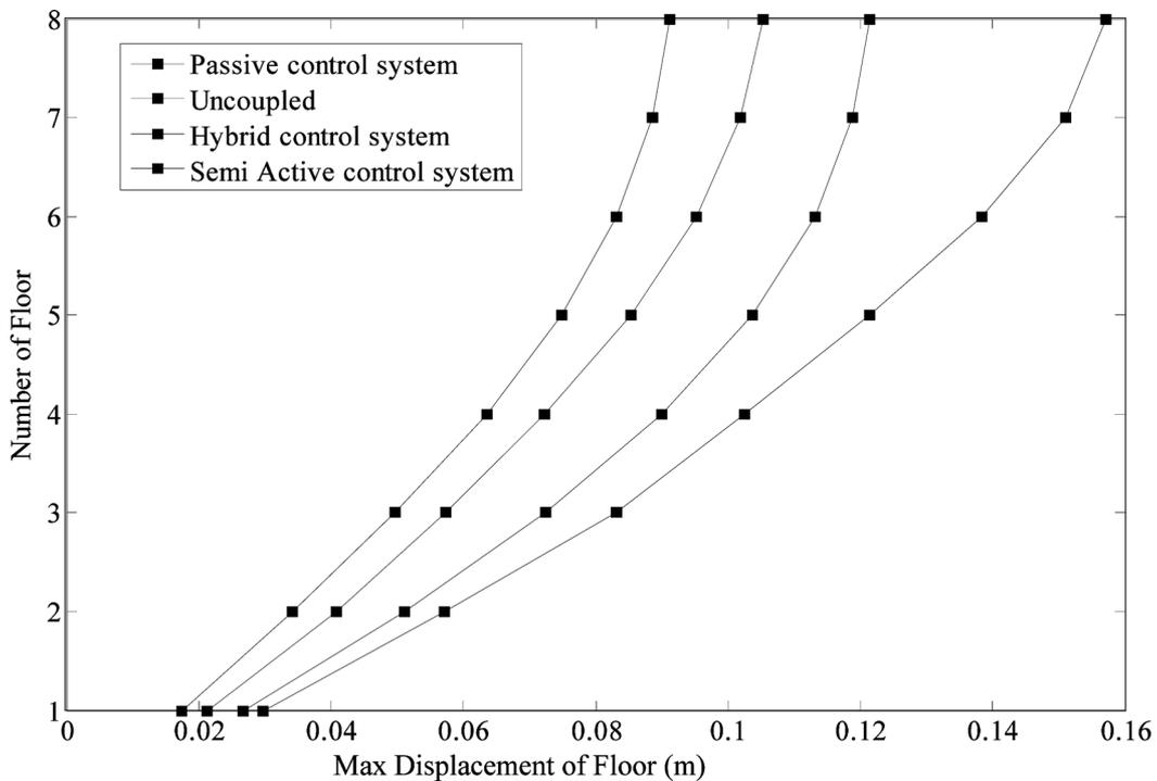
Fig. 9 Maximum displacement of stories of building 2 in different coupling configurations
