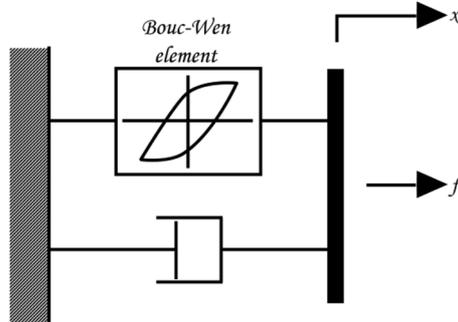
Fig. 2 Mechanical model of a shear mode type MR damper
