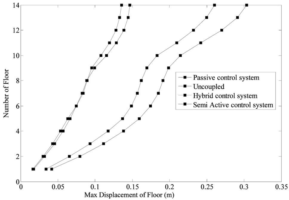
Fig. 7 Maximum displacement of stories of building 1 in different coupling configurations
