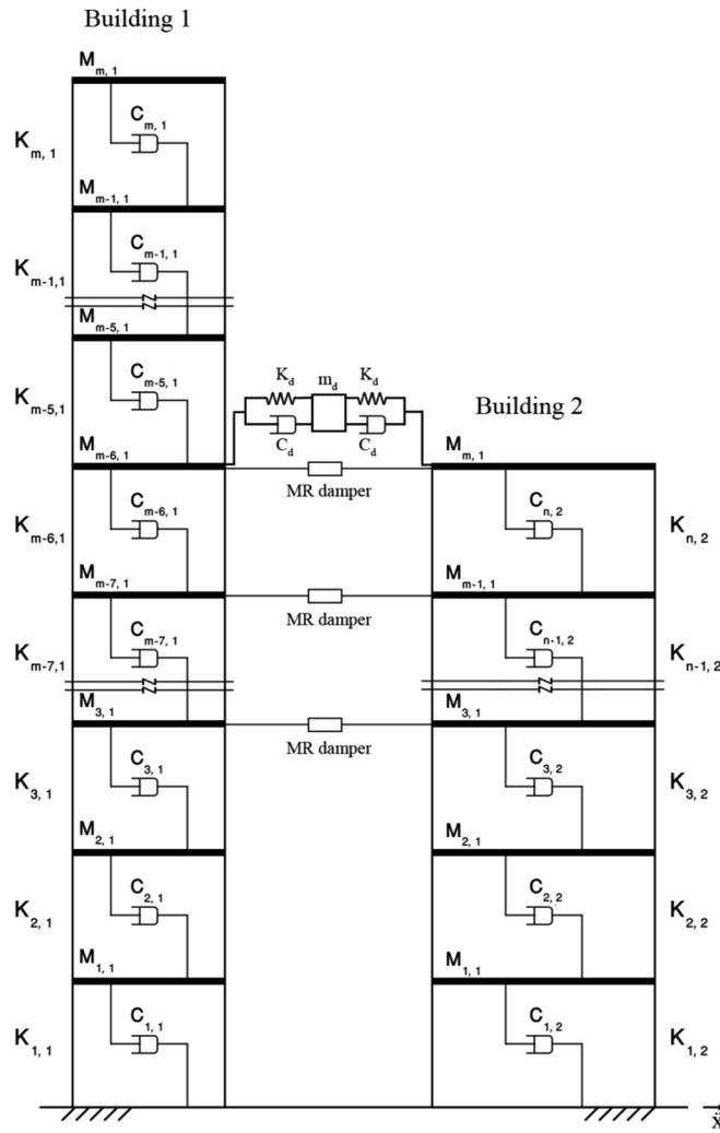
Fig. 1 Schematic diagram of a building complex with Magneto-Rheological Dampers and Tuned Mass Damper
