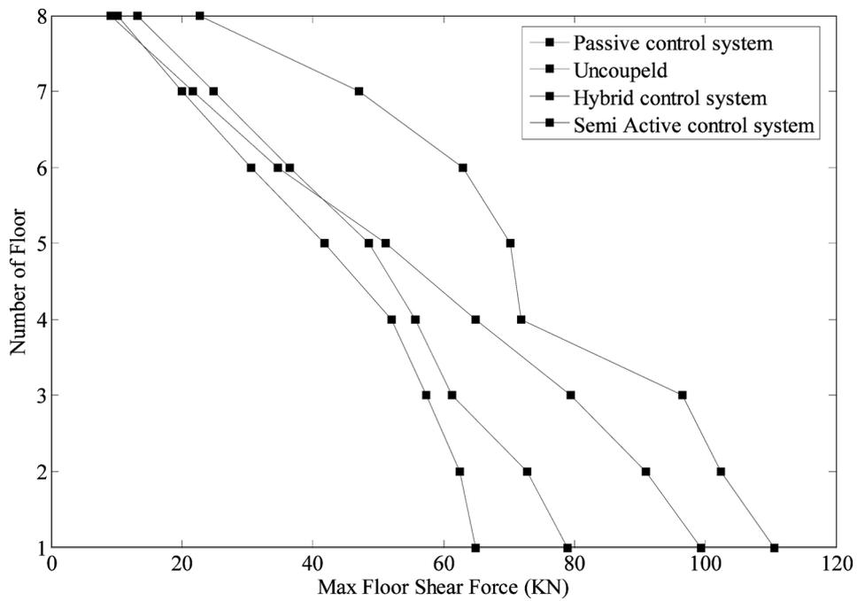
Fig. 8 Maximum shear force in different stories of building 2 in different coupling configurations
