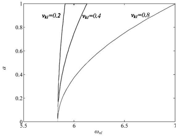
Fig. 4 Non-linear frequency-response curves for different slenderness coefficients.  $v_f = 0.8$ ,  $u_0 = 1$ ,  $u_1 = 0.1$ , 5 masses,  $\alpha = 0.1$
