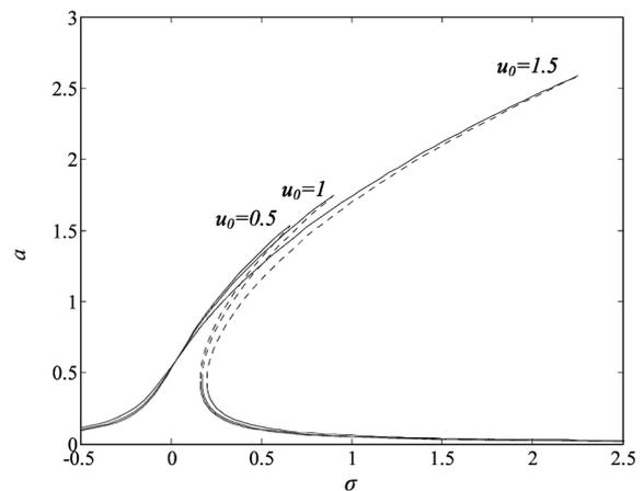
Fig. 9 Force-response curves for different mean axial velocities.  $v_f=0.8$ ,  $v_{kl}=0.4$  ( $v=L/2$ ),  $u_1=0.1$ ,  $m=5$  masses,  $\alpha=0.1$
