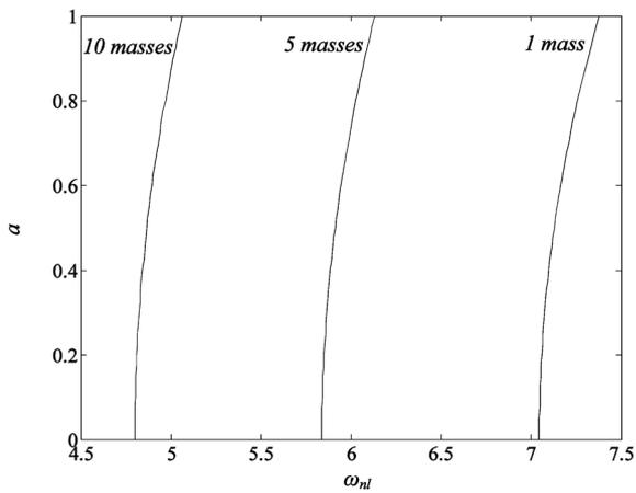
Fig. 6 Non-linear frequency-response curves for different mass numbers.  $v_f = 0.8$ ,  $v_{k1} = 0.4$  ( $v = L/2$ ),  $u_0 = 1$ ,  $u_1 = 0.1$ ,  $\alpha = 0.1$
