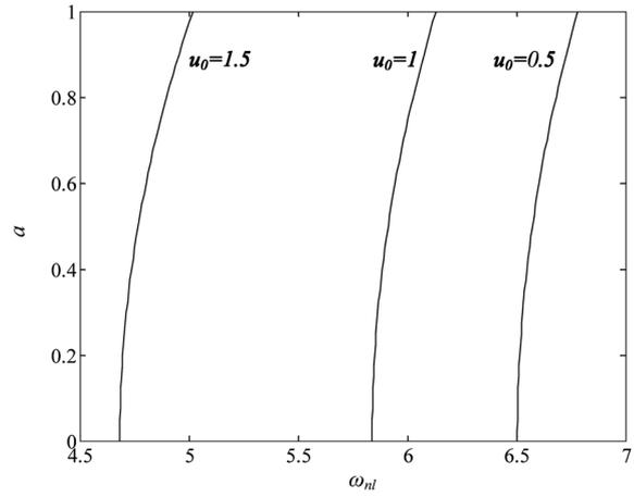
Fig. 5 Non-linear frequency-response curves for different mean axial velocities.  $v_f = 0.8$ ,  $v_{k1} = 0.4$  ( $v = L/2$ ),  $u_1 = 0.1$ , 5 masses,  $\alpha = 0.1$
