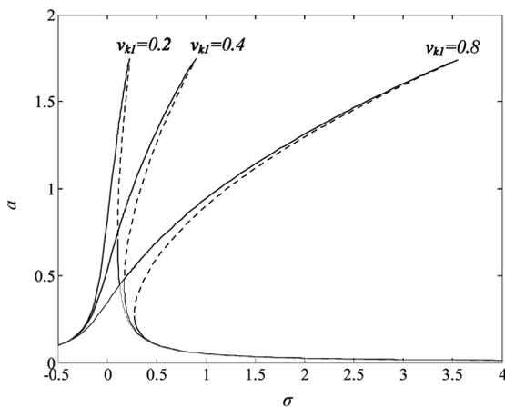
Fig. 8 Force-response curves for different slenderness coefficients.  $v_f=0.8$ ,  $u_0=1$ ,  $u_1=0.1$ ,  $m=5$  masses,  $\alpha=0.1$
