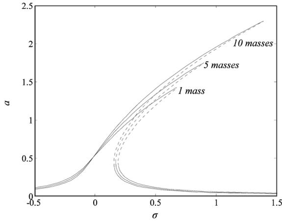
Fig. 10 Force-response curves for different mass numbers.  $v_f = 0.8$ ,  $v_{k1} = 0.4$  ( $v = L/2$ ),  $u_0 = 1$ ,  $u_1 = 0.1$ ,  $\alpha = 0.1$
