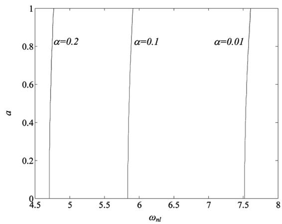
Fig. 7 Non-linear frequency-response curves for different mass ratios.  $v_f = 0.8$ ,  $v_{k1} = 0.2$  ( $v = L/4$ ),  $u_0 = 1$ ,  $u_1 = 0.1$ ,  $m = 5$  masses
