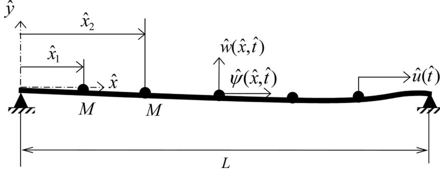
Fig. 1 Axially moving beam with multiple concentrated masses
