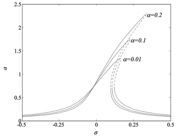
Fig. 11 Force-response curves for different mass ratios.  $v_f = 0.8$ ,  $v_{k1} = 0.2$  ( $v = L/4$ ),  $u_0 = 1$ ,  $u_1 = 0.1$ ,  $m = 5$  masses
