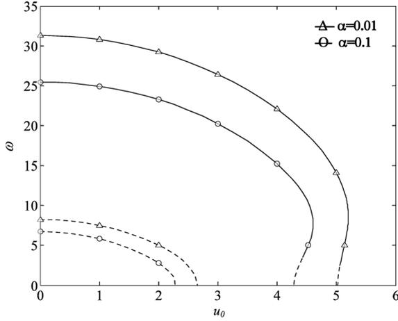
Fig. 2 Axial velocity versus natural frequency of the beam having 5 masses for different  $\alpha$  values,  $v_f = 0.8$  (dashed line: first mode, solid line: second mode)
