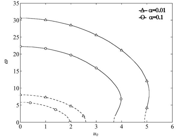
Fig. 3 Axial velocity versus natural frequency of the beam having 10 masses for different  $\alpha$  values,  $v_f = 0.8$  (dashed line: first mode, solid line: second mode)
