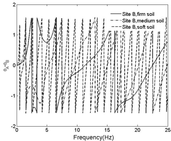
Fig. 12 Phase difference owing to seismic wave propagation through sites with different soil properties
