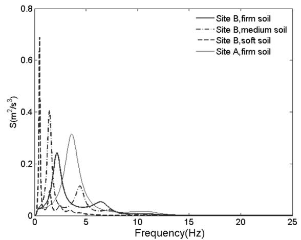
Fig. 11 Power spectral densities of ground motions at sites with different soil properties
