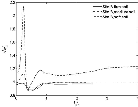
Fig. 14 Normalized total responses for different soil properties
