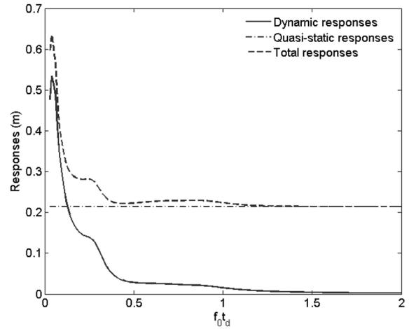
Fig. 15 Dynamic, quasi-static and total responses (medium soil at support B)
