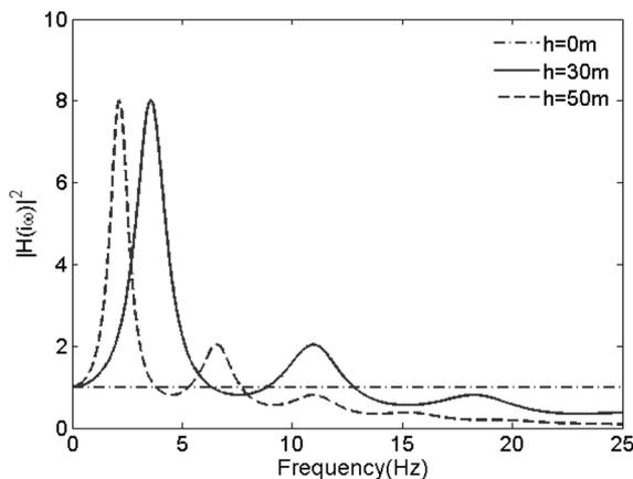
Fig. 4 Site transfer functions for different soil depths
