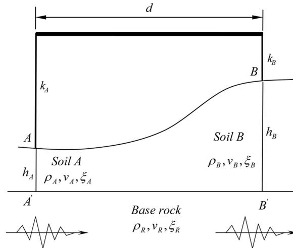
Fig. 1 Schematic view of a bridge frame crossing a canyon site
