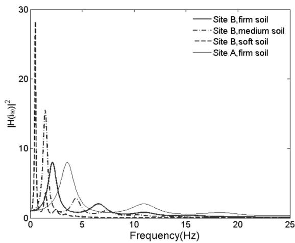
Fig. 10 Soil site transfer function for different soil properties
