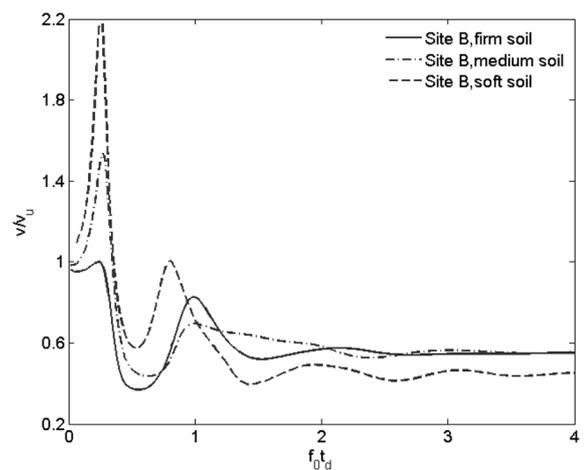
Fig. 13 Normalized dynamic responses for different soil properties
