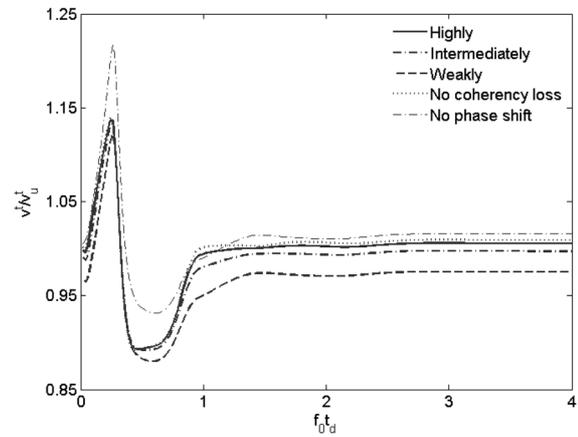
Fig. 17 Normalized total responses for different coherency losses
