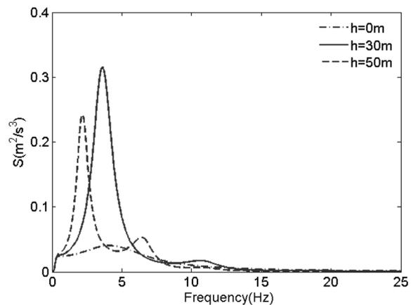
Fig. 5 Power spectral densities of ground motions on site of different depths
