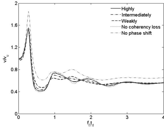
Fig. 16 Normalized dynamic responses for different coherency losses
