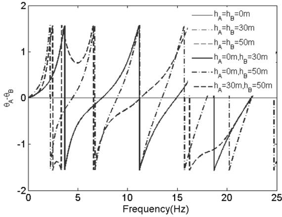
Fig. 6 Phase difference caused by seismic wave propagation through sites of different depths
