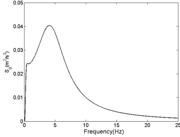
Fig. 2 Filtered ground motion power spectral density function on the base rock
