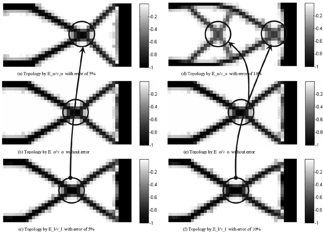
Fig. 5 Optimal topologies by considering the uncertainty error of 5% and 10% including a nominal optimal topology
