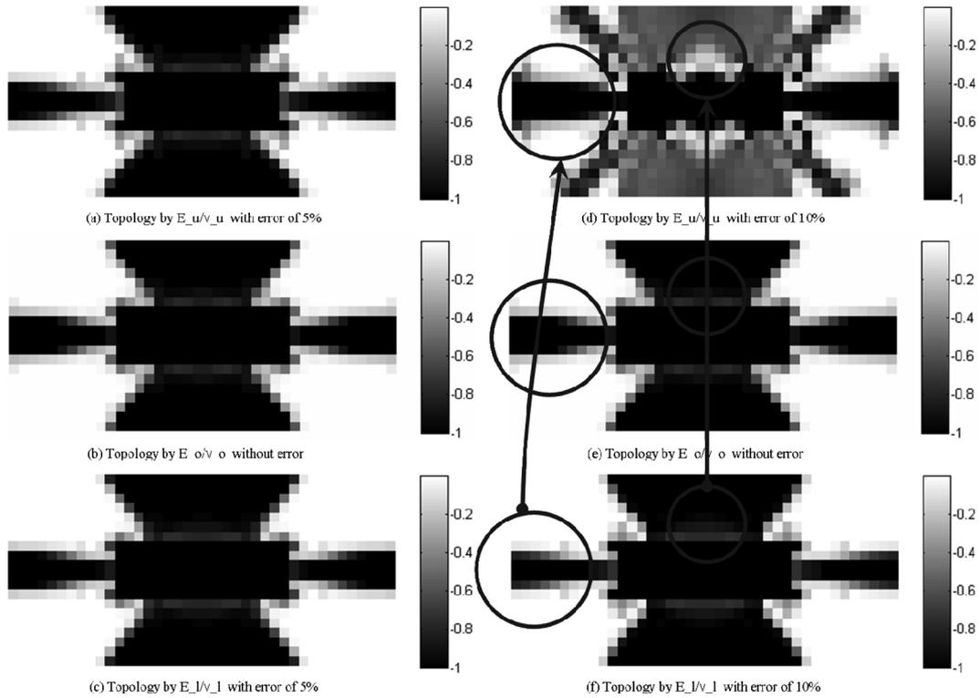
Fig. 9 Optimal topologies by considering the uncertainty error of 5% and 10% including a nominal optimal topology
