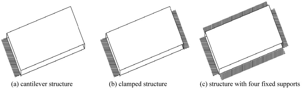
Fig. 4 Structural models
