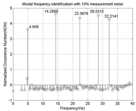
Fig. 5 **NON** of the system with 10% measurement noise
