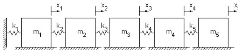
Fig. 1 The discrete mass-spring example
