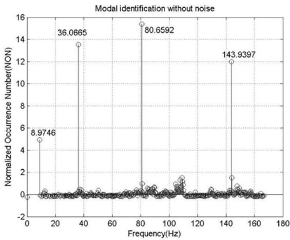
Fig. 7 NON of the beam model for noise-free measurements
