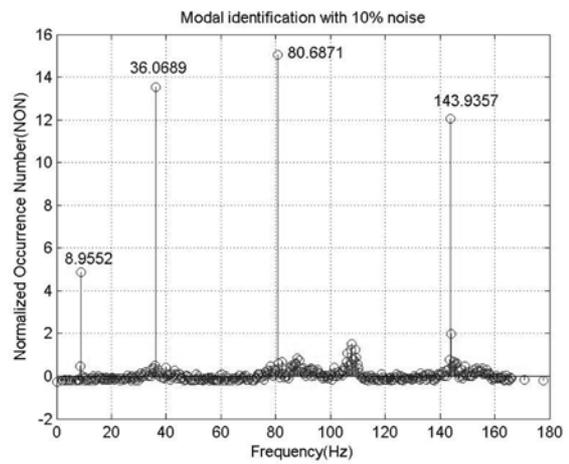
Fig. 8 NON of the beam model with 10% measurement noise
