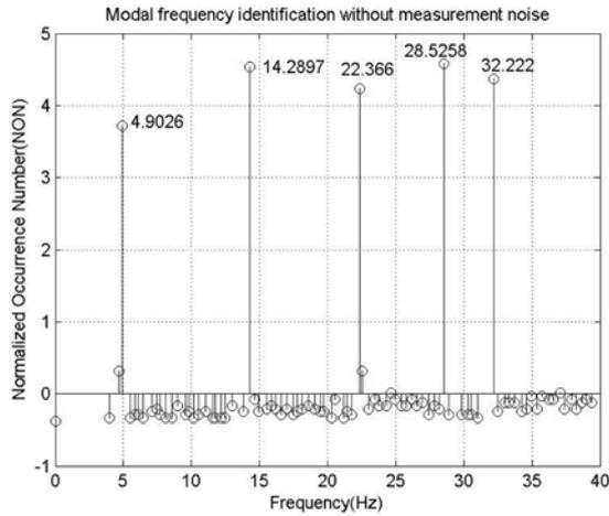
Fig. 4 **NON** of the system for noise-free measurements
