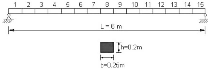
Fig. 6 The simulated simply supported beam
