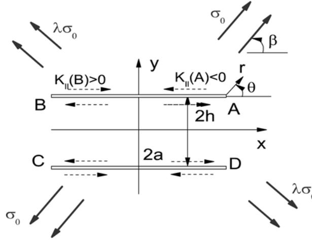
Fig. 1 Two parallel cracks of equal length  $2a$  and spaced by  $2h$  in an infinite elastic plane
