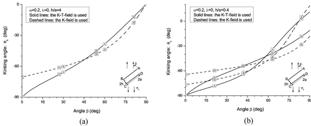
Fig. 3 Kinking angle at the crack tips A( $a, h$ ) and D( $a, -h$ ) versus the crack inclination angle  $\beta$  for two parallel cracks under simple uniaxial tension; (a)  $h/a = 4$ , (b)  $h/a = 0.4$
