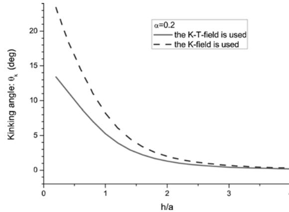
Fig. 2 The influence of the crack spacing on the kinking angle for the case of uniaxial mode I tensile loading
