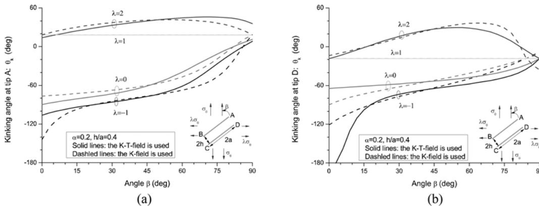
Fig. 5 Kinking angle versus crack inclination angle  $\beta$  for two parallel cracks with small spacing for different biaxiality ratios; (a) tip A( $a, h$ ), (b) tip D( $a, -h$ )
