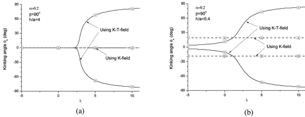
Fig. 6 Effect of the biaxiality ratio  $\lambda$  on the kinking angle at the crack tips A( $a, h$ ) and D( $a, -h$ ) versus  $\lambda$  with  $\beta = 90^\circ$ ,  $\alpha = 0.2$ ; (a)  $h/a = 4$ , (b)  $h/a = 0.4$
