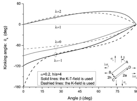
Fig. 4 Kinking angle at the crack tips A( $a, h$ ) and D( $a, -h$ ) versus the crack inclination angle  $\beta$  for two parallel cracks with large spacing for different biaxiality ratios
