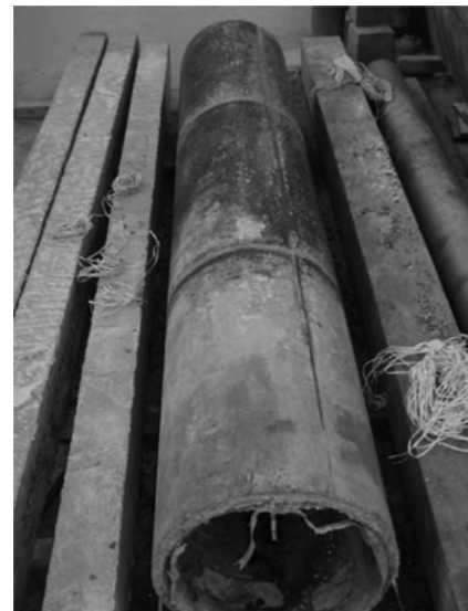
Fig. 4 Pipe after dismantling of moulds
