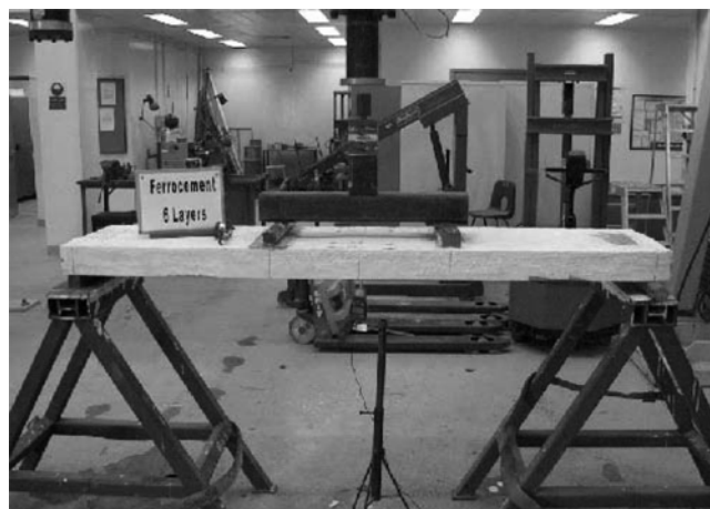
Fig. 18 Test rig and typical panel tested
