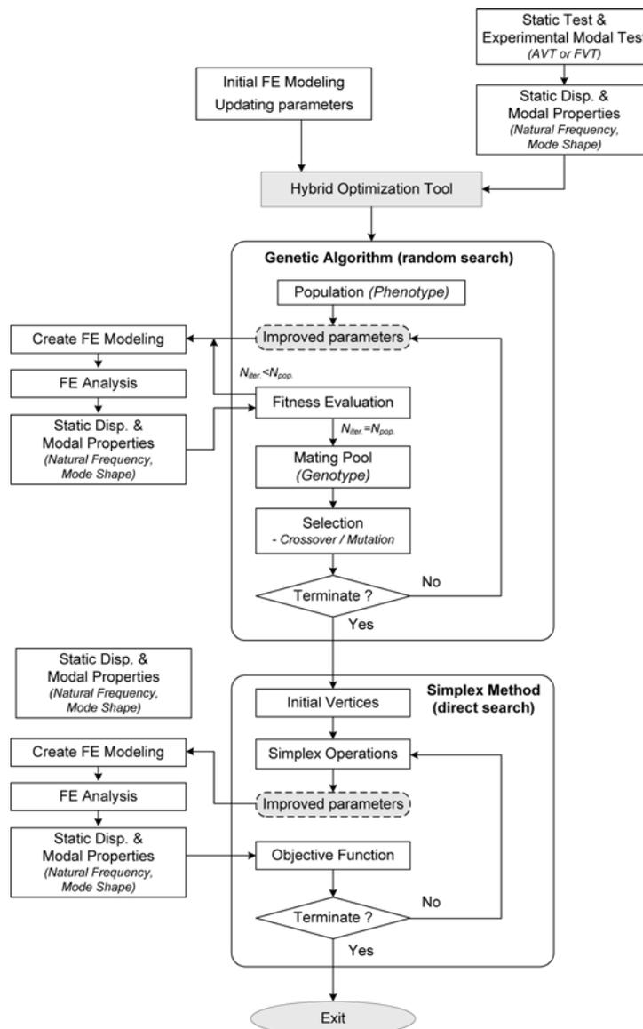
Fig. 1 Flowchart of the HGA based FE model updating method
