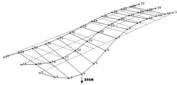
Fig. 8 Deformed shape under static load
