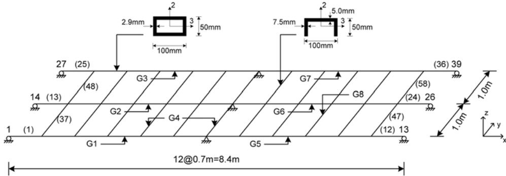
Fig. 7 Two span continuous grid model
