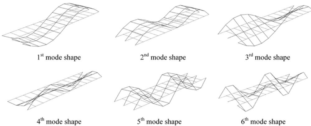
Fig. 9 Analytical mode shapes of the reference FE model
