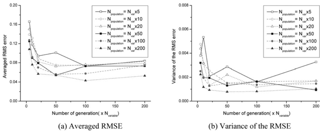
Fig. 6 Comparison of RMSE of updating variables according to the number of generation
