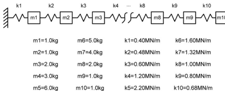
Fig. 2 The 10-DOF spring-mass system
