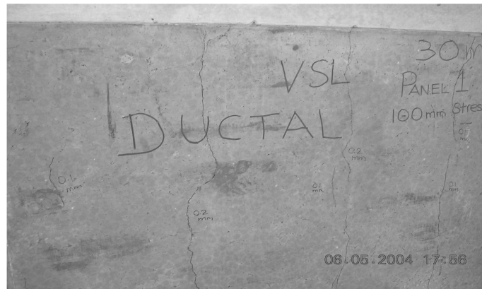
Fig. 14 Crack pattern of the UHSC Panel No.1
