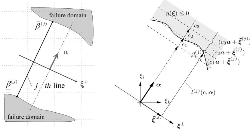
Fig. 1 Limit state and important direction  $\alpha$  for Line Sampling
