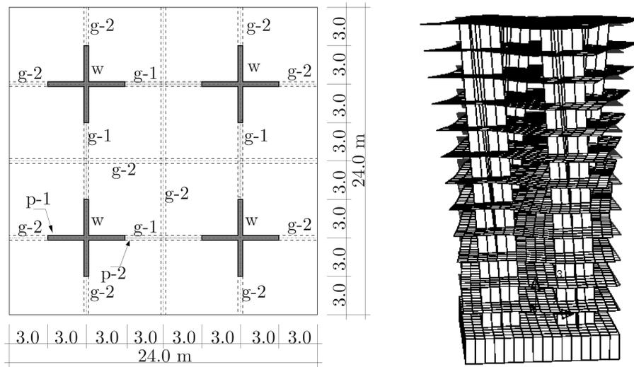
Fig. 2 Left: Floor plan of twelve story building supported by concrete walls (w) and girders of type g-1 and type g-2. Critical strains are considered at positions p-1 and p-2. Right: First mode shape of displacements
