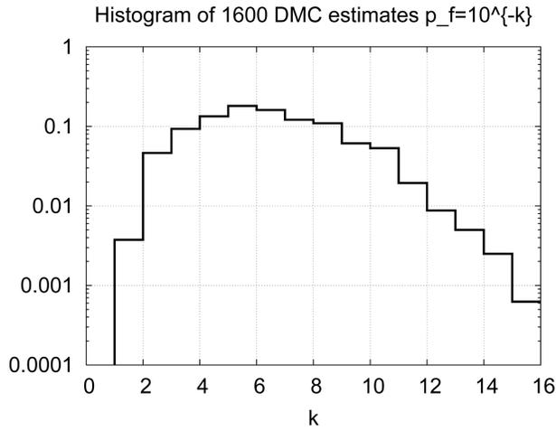
Fig. 3 Conditional failure probabilities by direct Monte Carlo sampling using a sample size of  $N = 1600$  lead to the mean  $\hat{p}_f = 0.00023$  with a standard deviation  $\sigma_{\hat{p}_f} = 0.000034$
