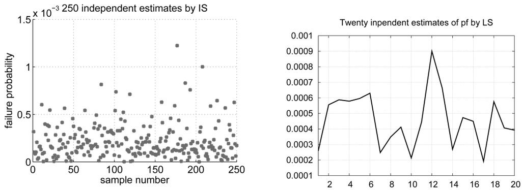
Fig. 4 Left: Conditional failure probabilities by Importance Sampling using a sample size of  $N = 250$  lead to the mean  $\hat{p}_f = 0.00023$  with a standard deviation  $\sigma_{\hat{p}_f} = 0.000012$ . Right: Twenty independent estimates of the total first excursion probability of the uncertain structure lead to the mean  $\hat{p}_f = 0.00046$  with a standard deviation  $\sigma_{\hat{p}_f} = 0.000040$
