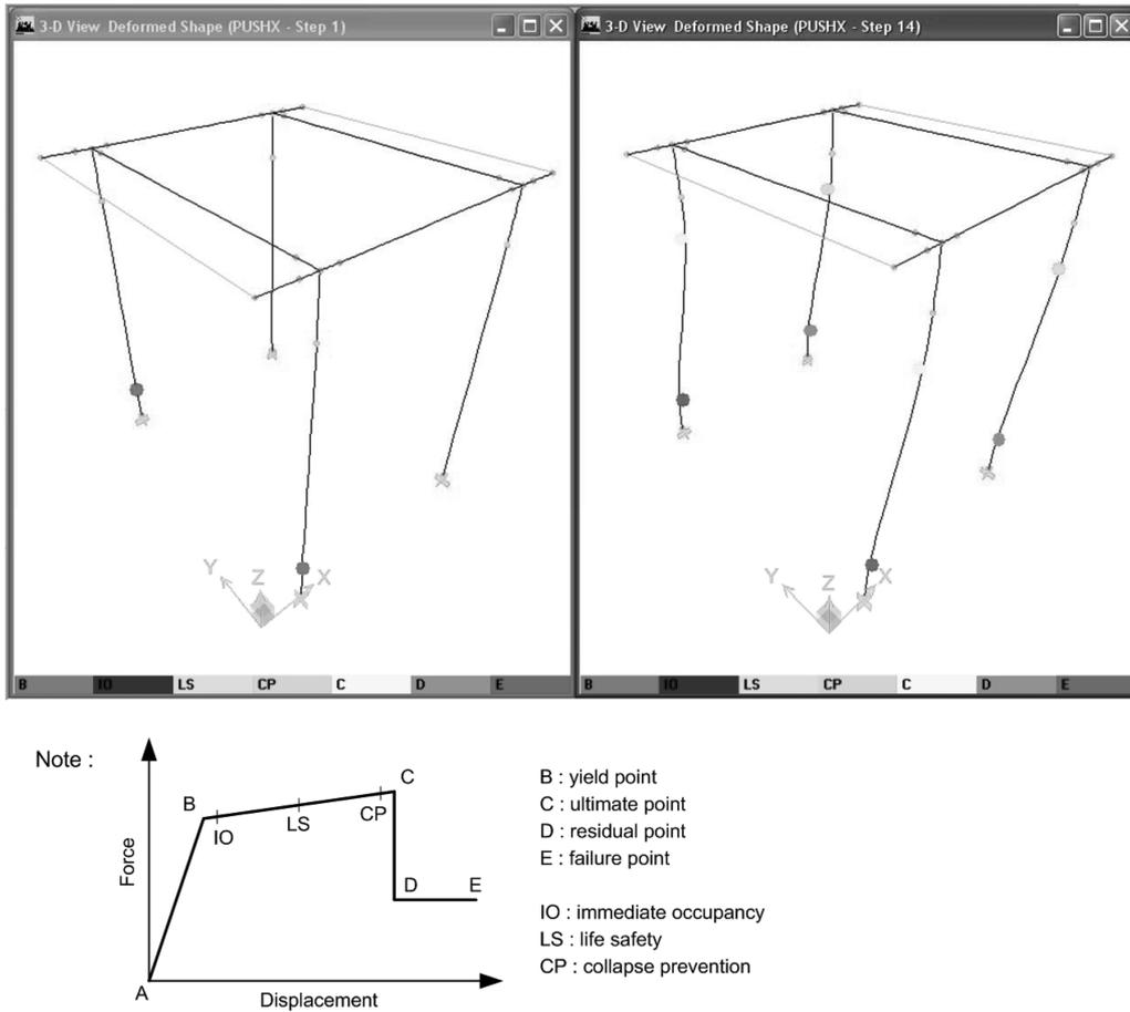
Fig. 9 Plastic hinge distribution on the first and last step of a pushover analysis of a simple reinforced concrete structure using ETABS
