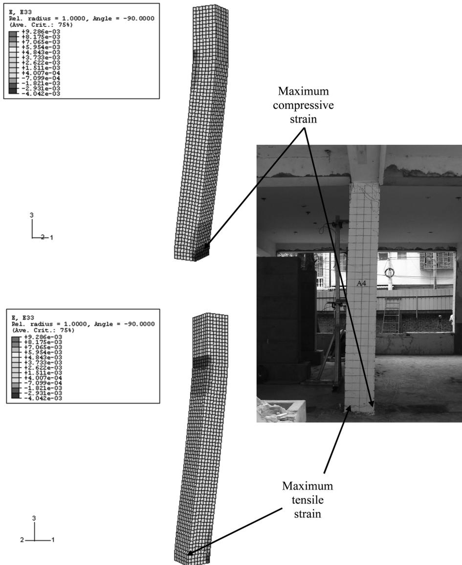
Fig. 16 Comparison of the RCM simulated response of an ordinary column and photograph of the actual Reuipu Elementary School building
