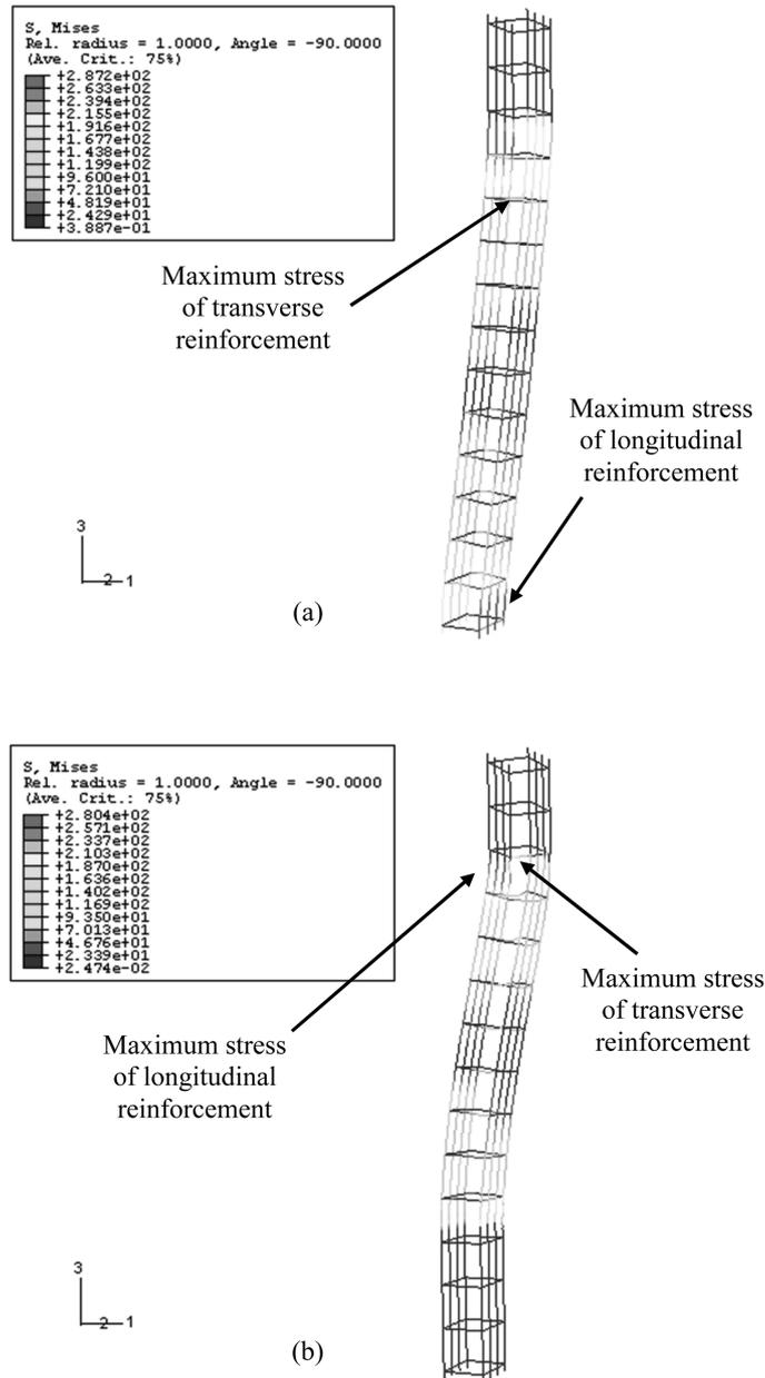
Fig. 18 RCM simulated response of a steel bar within (a) an ordinary column and (b) a captive column, as found in Reuipu Elementary School building
