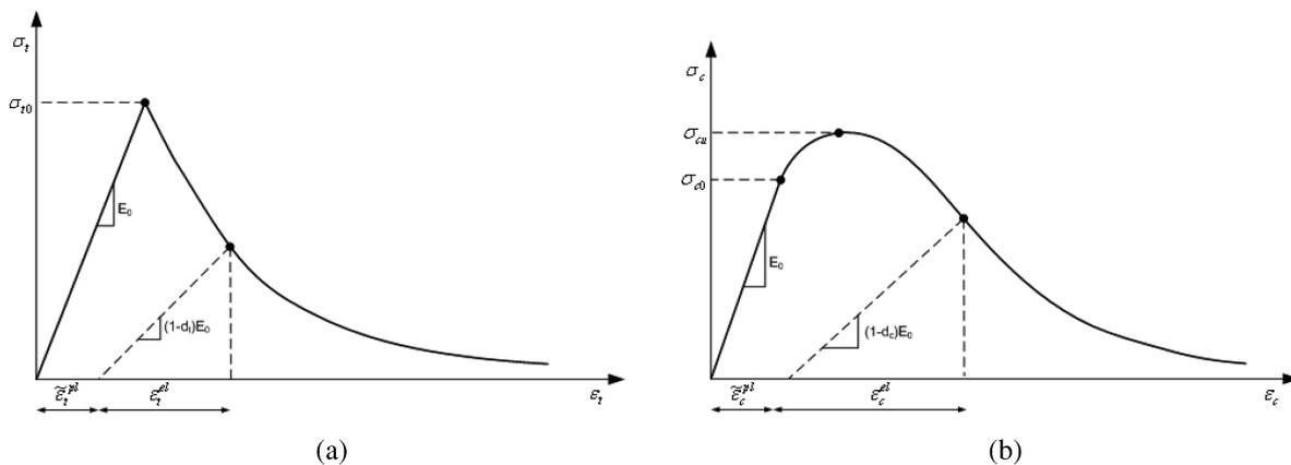
Fig. 2 Response of concrete subjected to uniaxial loading: (a) tension loading and (b) compression loading (ABAQUS 2004).
