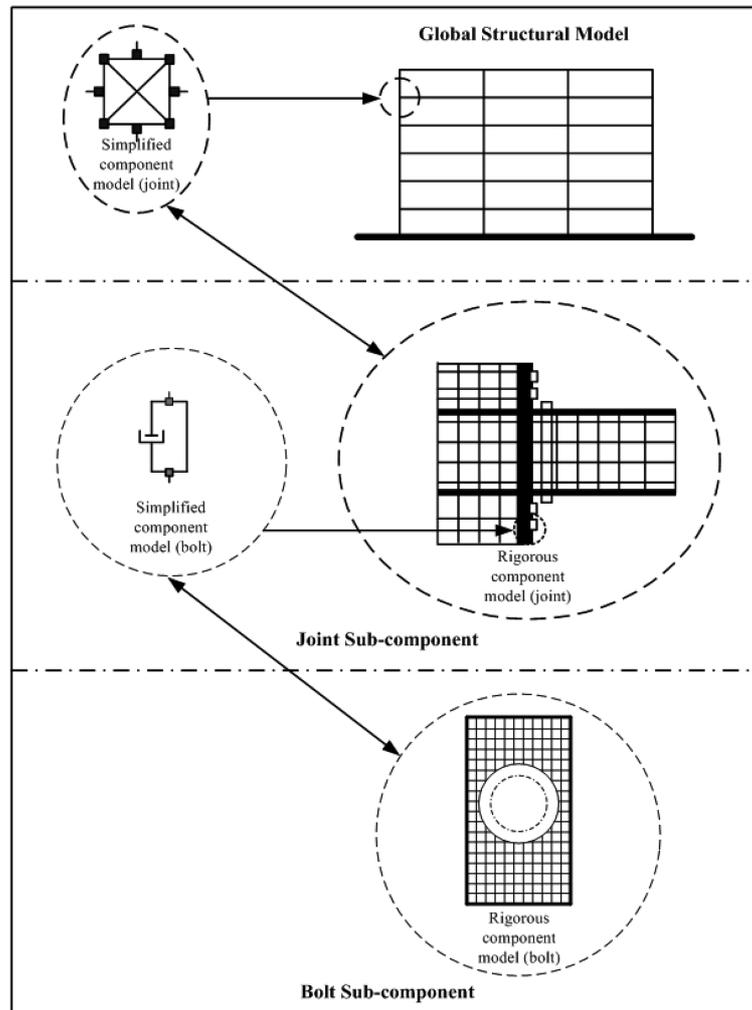
Fig. 1 Multi-level modeling and simulation method
