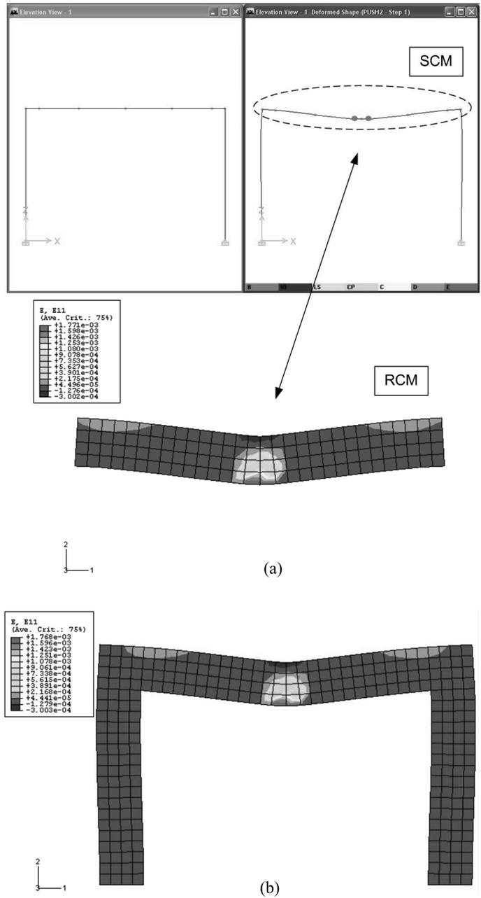
Fig. 6 The 2D portal frame model: (a) global frame model (SCM) and RCM simulated response of beam component using proposed method, (b) response of detailed portal frame model
