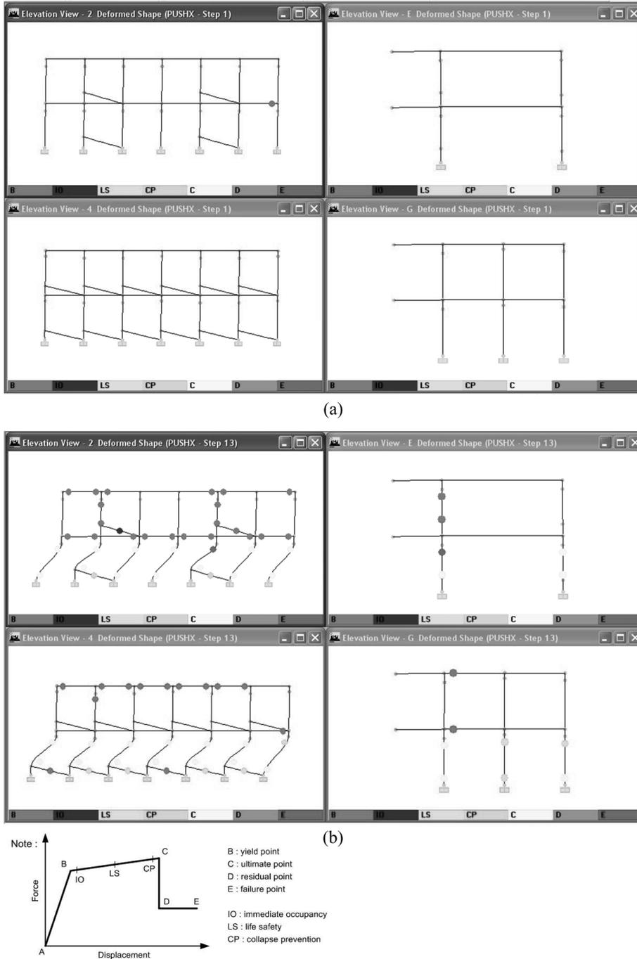
Fig. 14 Reuipu Elementary School building plastic hinge distribution of the pushover analysis using ETABS: (a) first step and (b) last step
