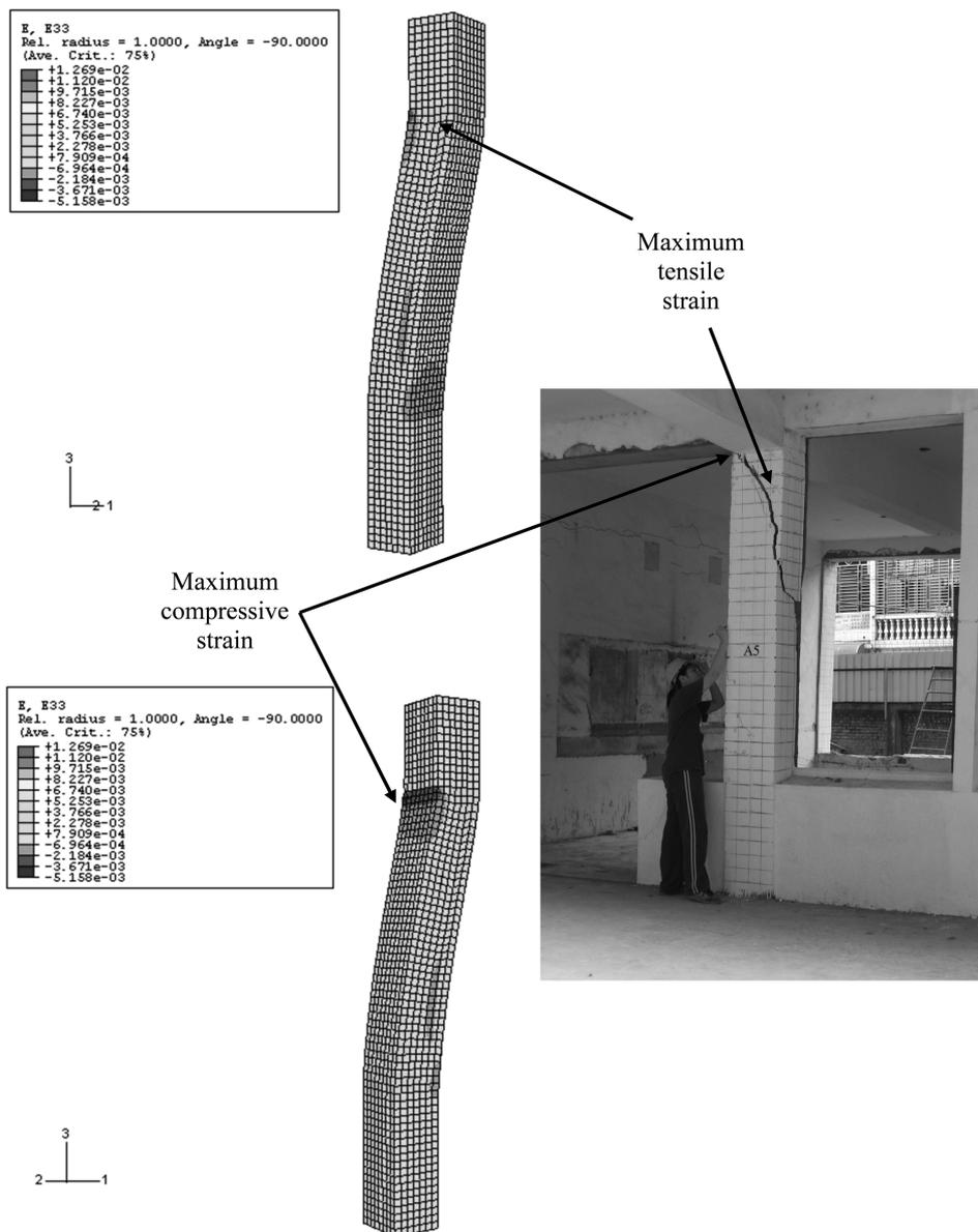
Fig. 17 Comparison of the RCM simulated response of a captive column and photograph of the actual Reuipu Elementary School building
