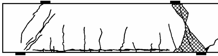
Fig. 8 Crack patterns at failure of specimen 'H4100'
