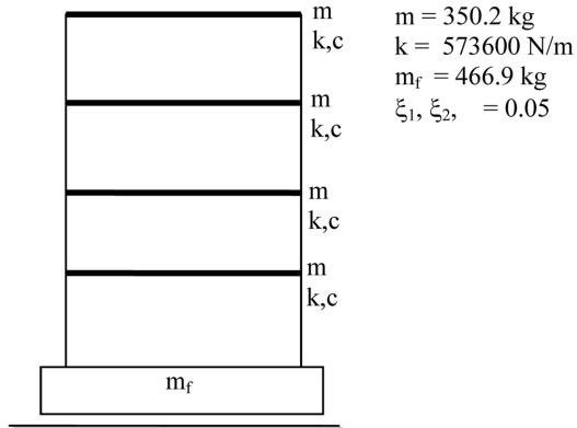
Fig. 1(a) Four story plane frame structure
