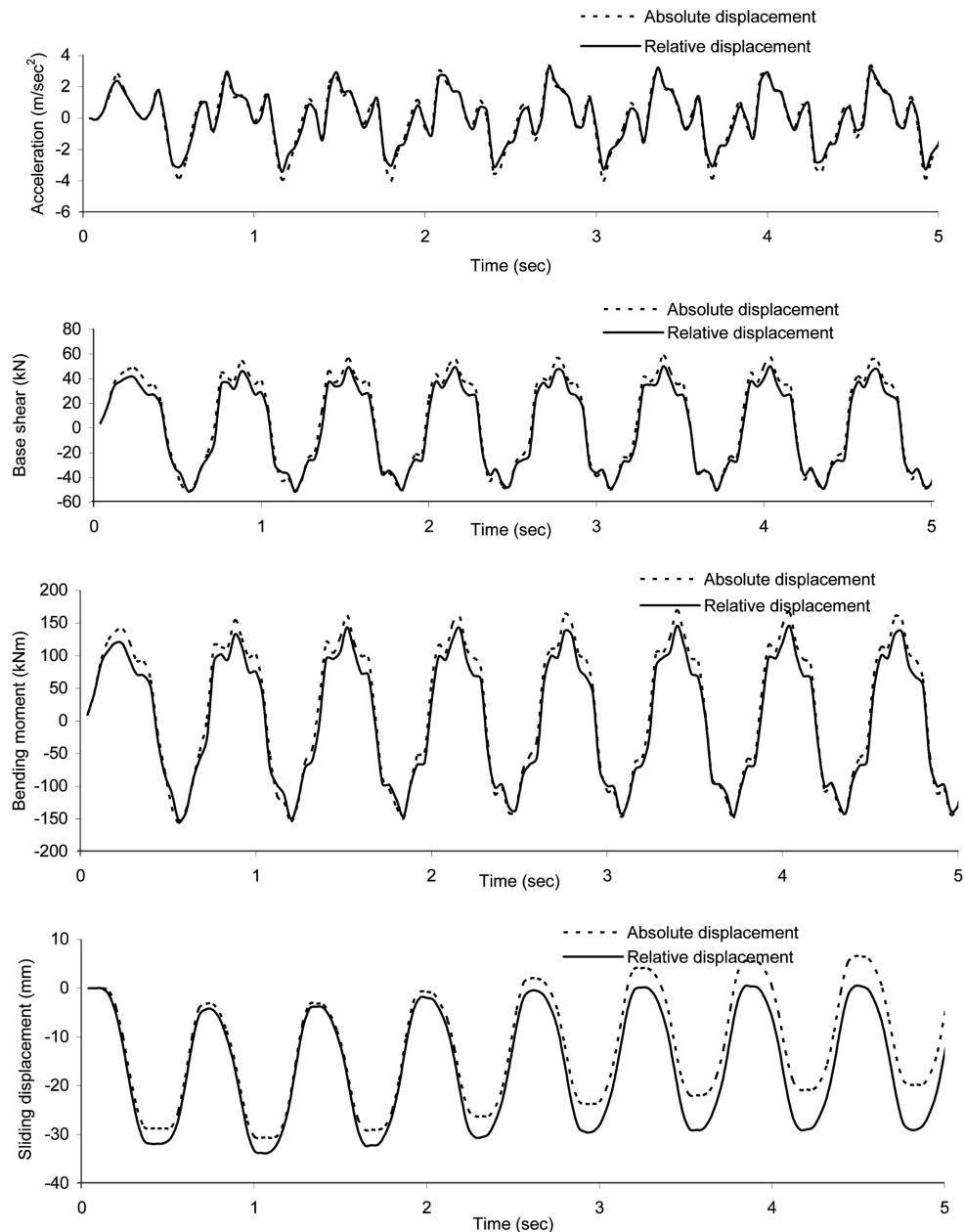
Fig. 3 Response of a four storey space frame structure subjected to harmonic ground acceleration
