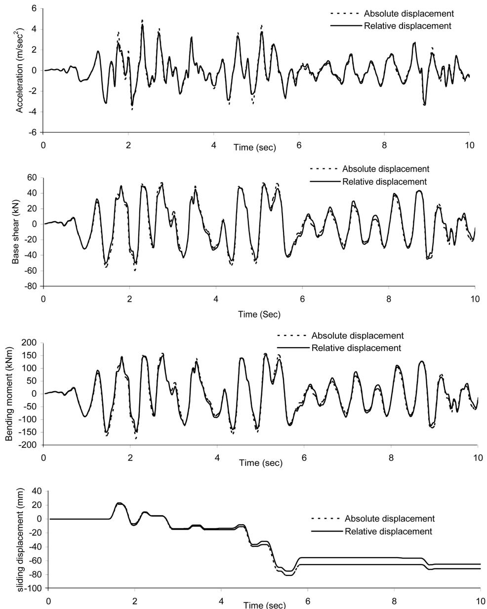
Fig. 4 Response of a four storey space frame structure subjected to earthquake ground acceleration
