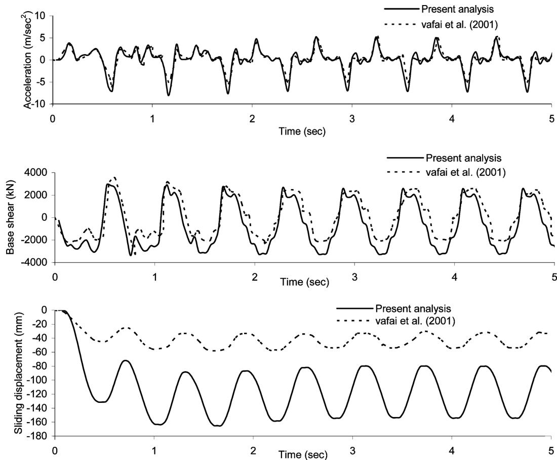
Fig. 2(b) Response of a four storey plane frame structure isolated at base
