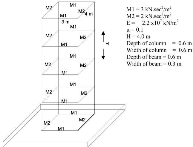
Fig. 1(b) Four story space frame structure
