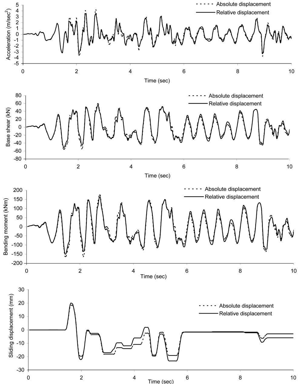
Fig. 5 Response of a four storey space frame structure with restoring force device subjected to earthquake ground acceleration
