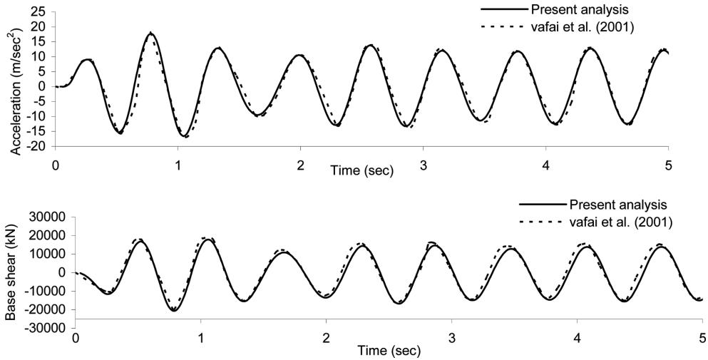
Fig. 2(a) Response of a four storey plane frame structure fixed at base
