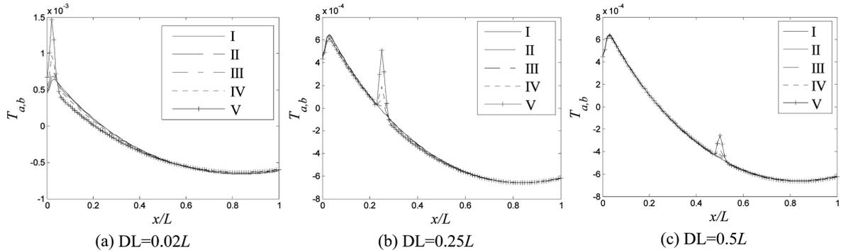
Fig. 2 Variation of wavelet coefficients wrt damage location and extent. I:  $D = 0$ , II:  $D = 20$ , III:  $D = 40$ , IV:  $D = 60$ , V:  $D = 80$ . Scale parameter:  $a = 3$ , DL: Damage Location,  $d = 0.5b_f + e$
