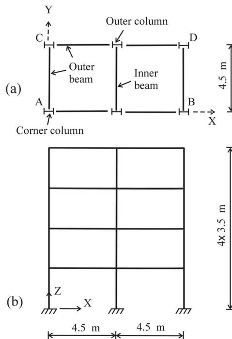
Fig. 2 Four-storey 52-member space frame: (a) plan, (b) side view
