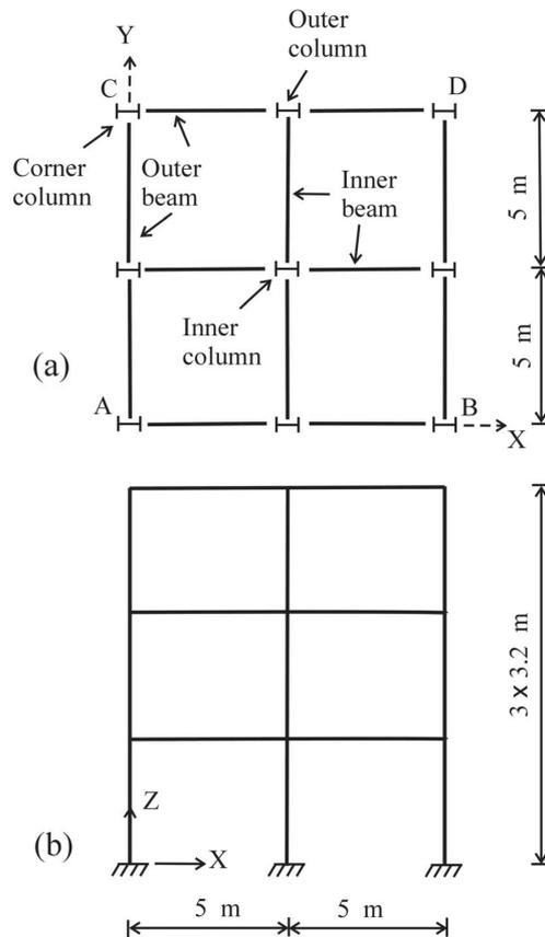
Fig. 3 Three-storey 63-member space frame: (a) plan, (b) side view
