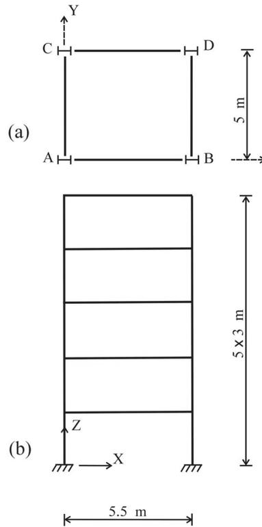
Fig. 1 Five-storey 40-member space frame: (a) plan, (b) side view
