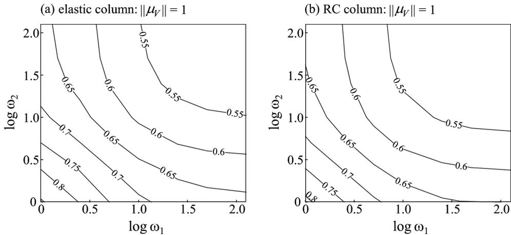
Fig. 11 Variation of effective length factor  $\alpha$  with respect to  $\log \omega_1$  and  $\log \omega_2$  of reinforced concrete columns RCC ( $\|\mu_V\| = 1$ ): (a) elastic constitutive relations for concrete, with reinforcement being neglected, and (b) non-linear constitutive relations for both concrete and steel
