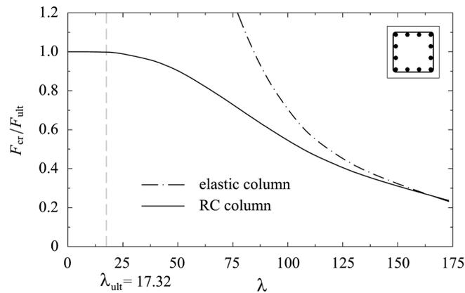
Fig. 6 The variation of normalized buckling load  $F_{cr}/F_{ult}$  vs. column slenderness  $\lambda$
