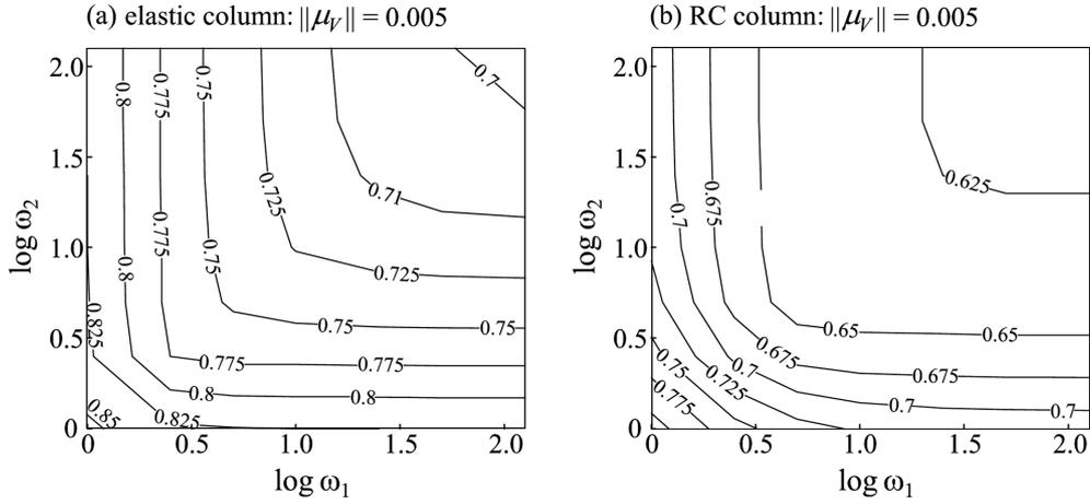
Fig. 10 Variation of effective length factor  $\alpha$  with respect to  $\log \omega_1$  and  $\log \omega_2$  for reinforced concrete columns RCB ( $\|\mu_V\| = 0.005$ ): (a) elastic constitutive relations for concrete, with reinforcement being neglected, and (b) non-linear constitutive relations for both concrete and steel
