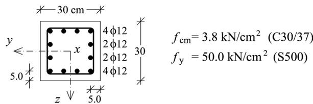
Fig. 3 Reference reinforced concrete cross-section. Geometric and material data
