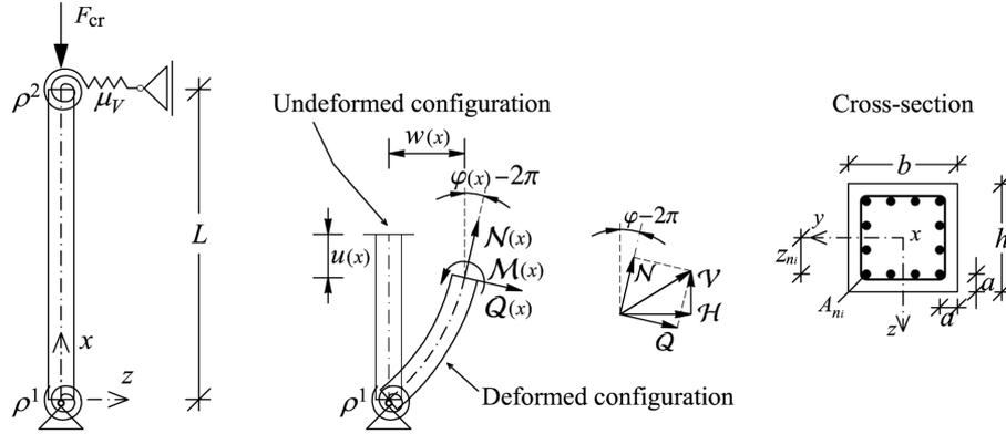
Fig. 1 Deformed and undeformed configuration of a restrained RC column. Reinforced concrete cross-section
