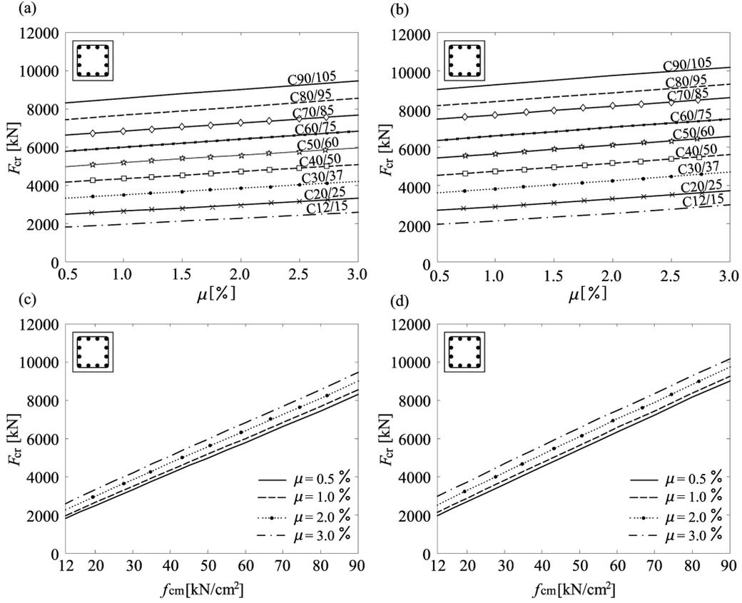
Fig. 7 The effect of the steel/concrete area ratio and strength of concrete on buckling load  $F_{cr}$ . (a) and (c) pinned-pinned column (PPC); (b) and (d) fixed-fixed column (FFC)
