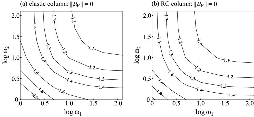
Fig. 9 Variation of effective length factor  $\alpha$  with respect to  $\log \omega_1$  and  $\log \omega_2$  for reinforced concrete columns RCA ( $\mu_V = 0$ ): (a) elastic constitutive relations for concrete, with reinforcement being neglected, and (b) non-linear constitutive relations for both concrete and steel
