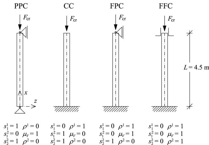
Fig. 5 Euler's reinforced concrete columns
