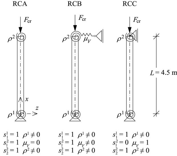
Fig. 8 Reinforced concrete columns with end restraints
