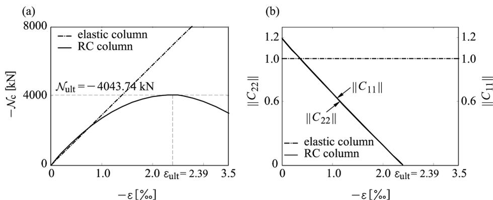
Fig. 4 The variations of (a) constitutive axial force  $N_c$  and (b) normalized flexural tangent stiffness  $\|C_{22}\| = C_{22}/E_{cm}J_c$  and normalized axial tangent stiffness  $\|C_{11}\| = C_{11}/E_{cm}A_c$  with respect to membrane deformation  $\varepsilon$
