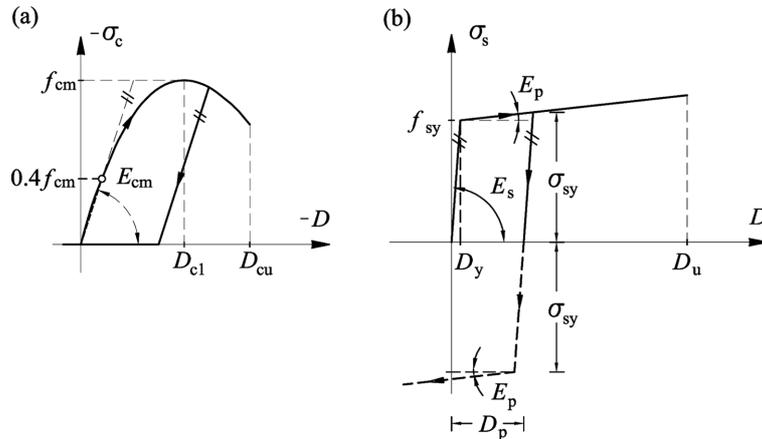
Fig. 2 Constitutive laws of (a) concrete and (b) reinforcing steel according to Eurocode 2 (2002)
