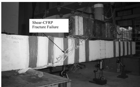
Fig. 3(c) Shear with CFRP fracture failure pattern for precracked/repaired specimen BS1-2
