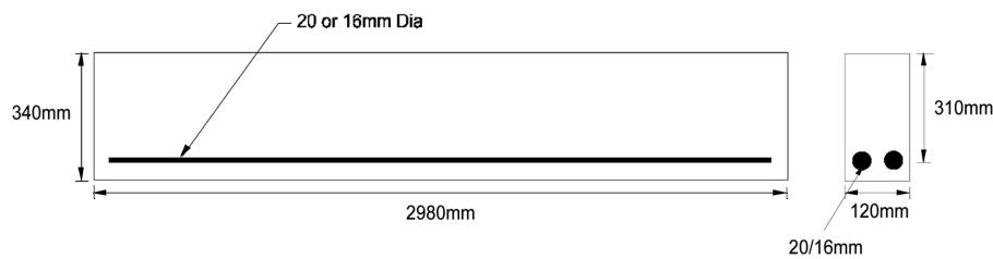
Fig. 1 Reinforcement details of series BT1/BT2/BS1/BS2
