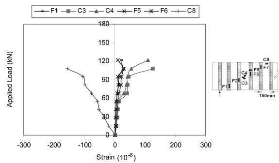
Fig. 5(b) Load versus surface strain in CFRP strip and concrete surface for precracked/repaired specimen BS1-1
