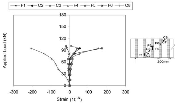
Fig. 5(c) Load versus surface strain in CFRP strip and concrete surface for precracked/repaired specimen BS1-2
