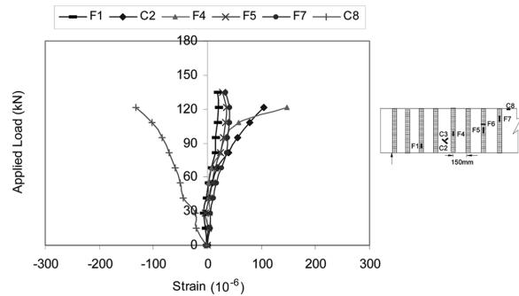
Fig. 5(d) Load versus surface strain in CFRP strip and concrete surface for precracked/repaired specimen BT2-1
