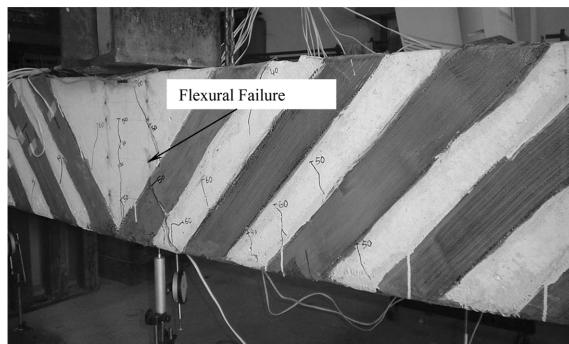
Fig. 3(g) Flexural failure pattern for precracked/repaired specimen BS2-2
