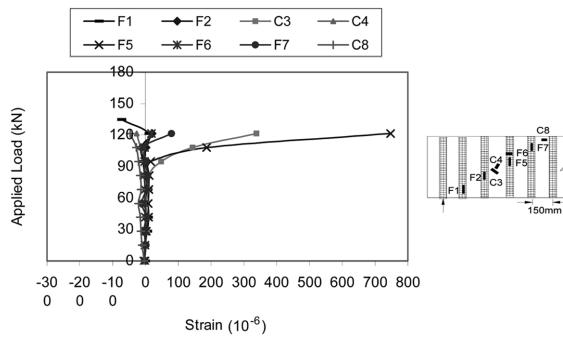
Fig. 5(a) Load versus surface strain in CFRP strip and concrete surface for precracked/repaired specimen BT1-1
