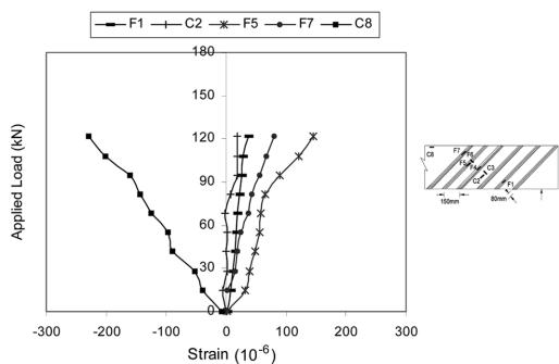
Fig. 5(e) Load versus surface strain in CFRP strip and concrete surface for precracked/repaired specimen BT2-2
