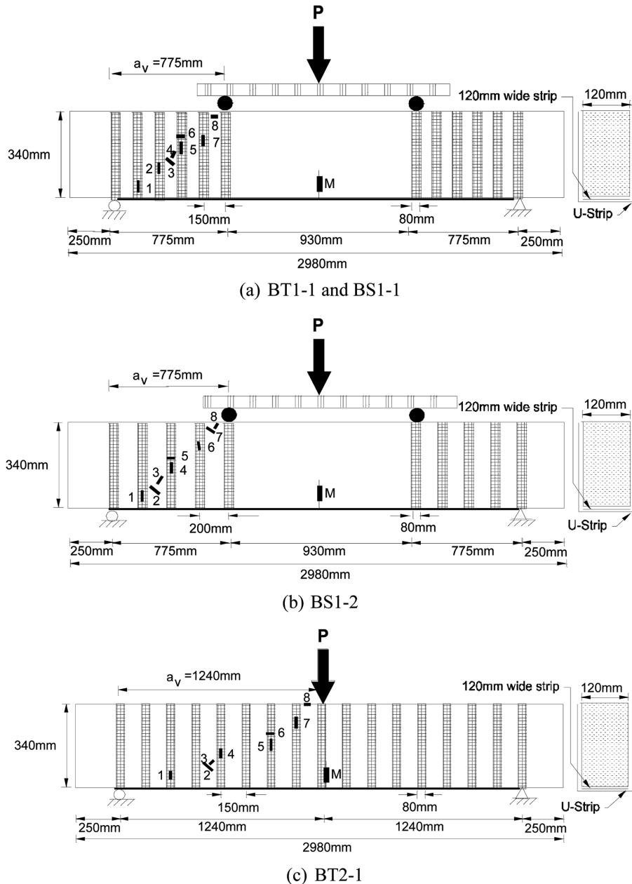
Fig. 2(a), (b), (c), (d), and (e): Strengthening patterns and test set-up
