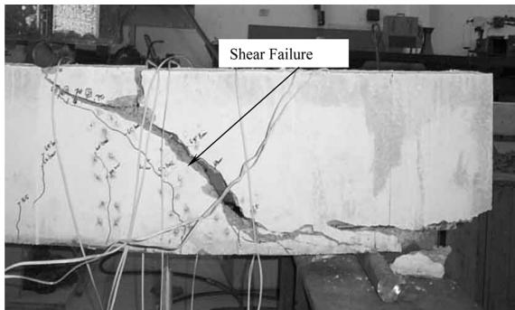
Fig. 3(a) Shear failure pattern for control specimen BT1a
