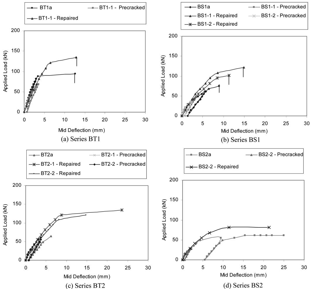
Fig. 4 (a), 4(b), 4(c), and 4(d): Load versus mid deflection curves of specimens in series BT1, BS1, BT2 and BS2
