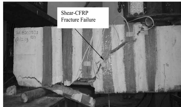
Fig. 3(b) Shear with CFRP fracture failure pattern for precracked/repaired specimen BT1-1
