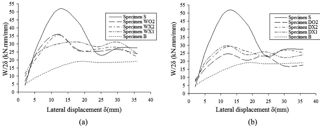
Fig. 14 Reduced energy dissipation per cycle divided by the corresponding displacement  $2$  of the cycle; (a) Window openings of various locations, (b) Door openings of various locations
