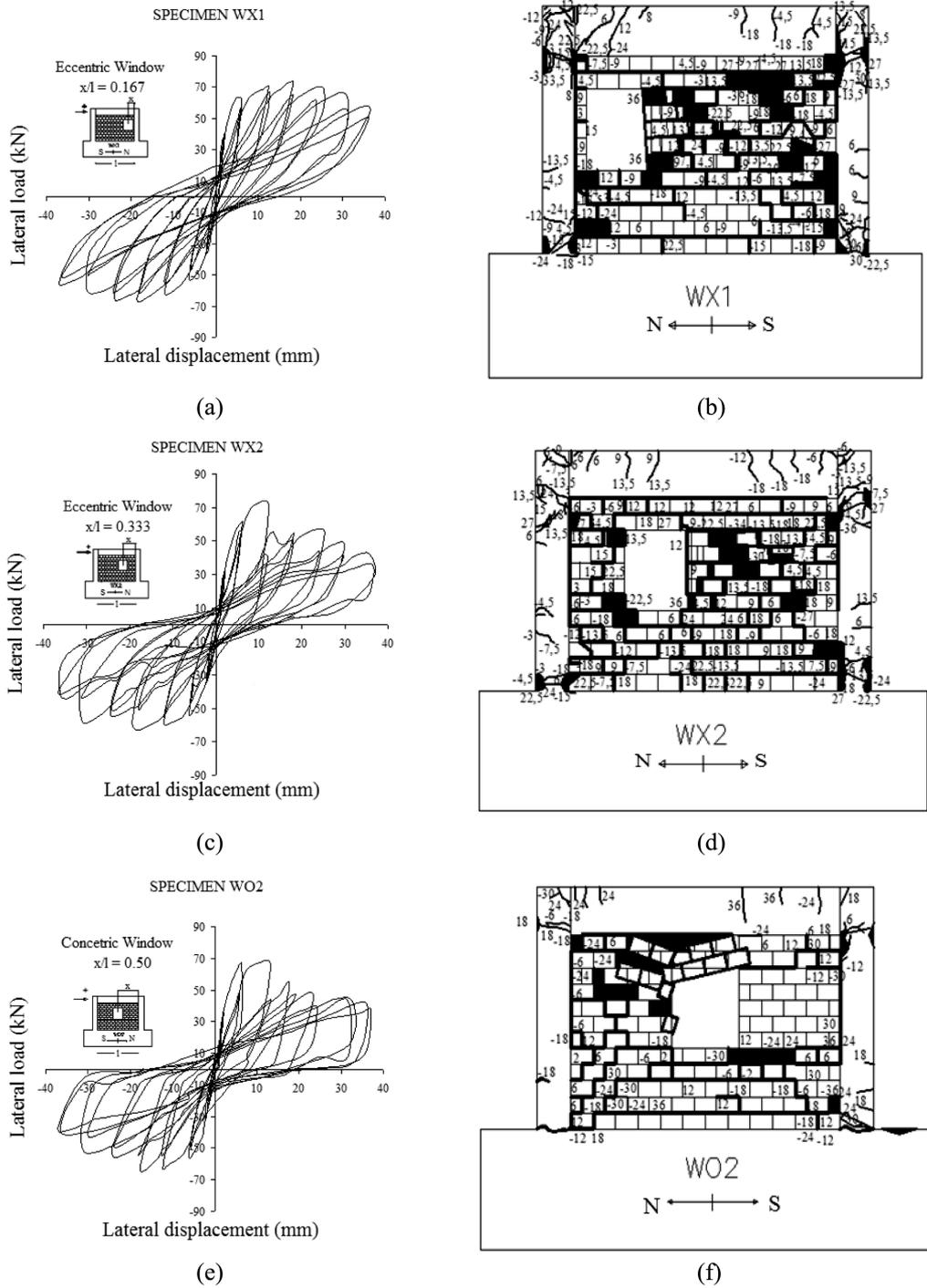
Fig. 7 Lateral load against displacement hysteresis curves and failure modes of infilled frame specimens with window openings and various opening locations, (a) and (b)  $x/l = 0.17$ , (c) and (d)  $x/l = 0.33$ , (e) and (f)  $x/l = 0.5$
