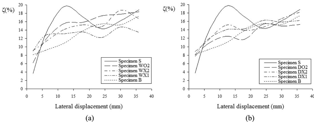
Fig. 15 Equivalent viscous damping ratio during the loading cycles; (a) Window openings of various locations, (b) Door openings of various locations
