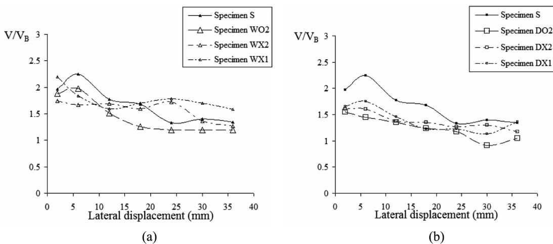
Fig. 12 Strength of the infilled frames over the strength of the corresponding bare frame; (a) Window openings of various locations, (b) Door openings of various locations
