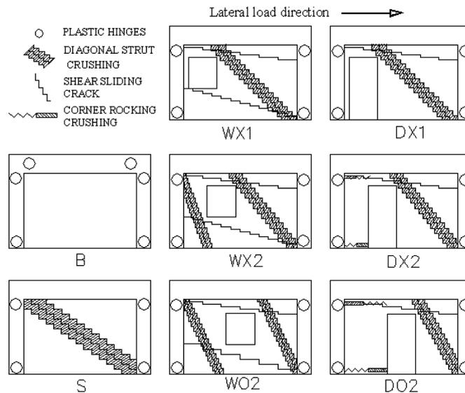
Fig. 9 Collapse mechanisms
