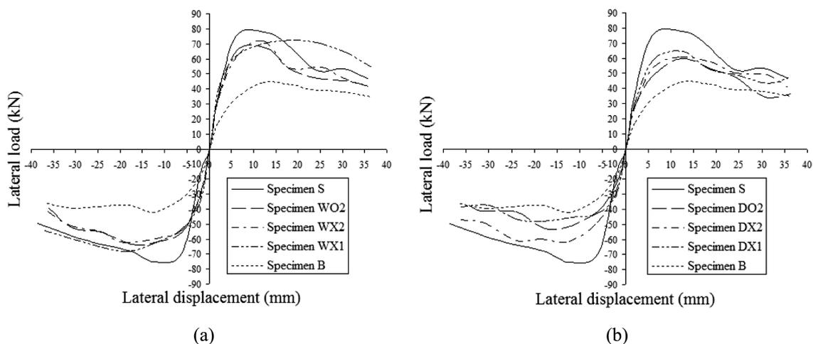
Fig. 10 Lateral load against displacement envelopes; (a) Window openings of various locations, (b) Door openings of various locations
