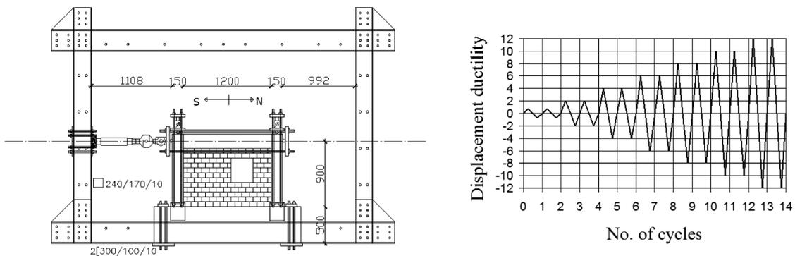
Fig. 3 Test setup (mm) and loading programme
