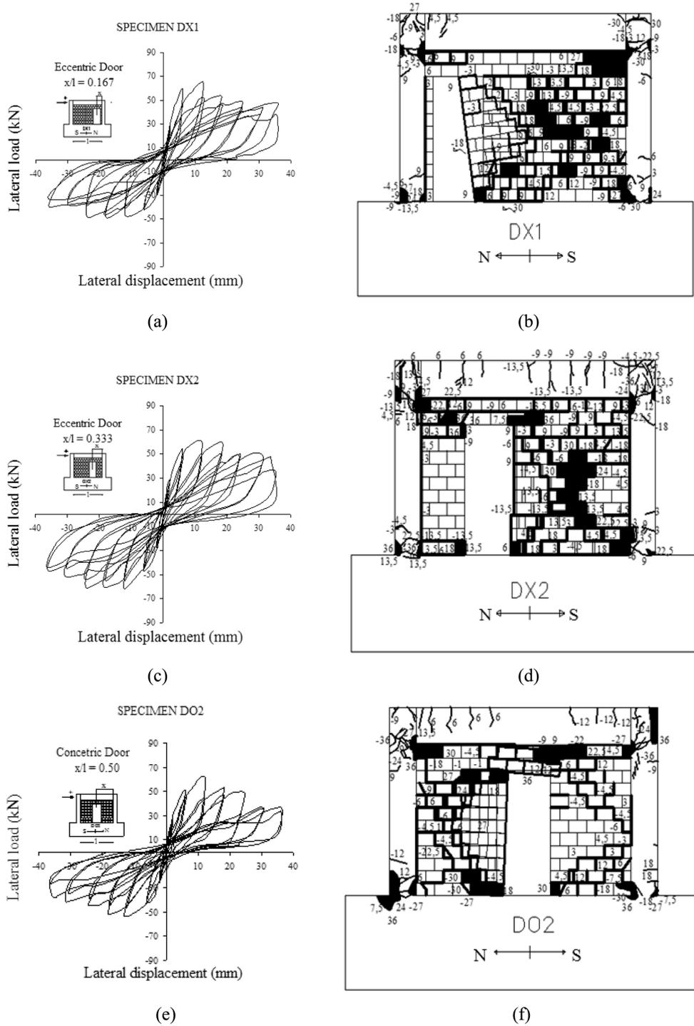
Fig. 8 Lateral load against displacement hysteresis curves and failure modes of infilled frame specimens with door openings and various opening locations, (a) and (b)  $x/l = 0.17$ , (c) and (d)  $x/l = 0.33$ , (e) and (f)  $x/l = 0.5$
