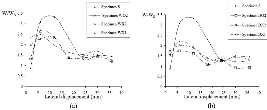
Fig. 13 Reduced energy dissipation capacity of the infilled frames over the reduced energy dissipation capacity of the corresponding bare frames; (a) Window openings of various locations, (b) Door openings of various locations
