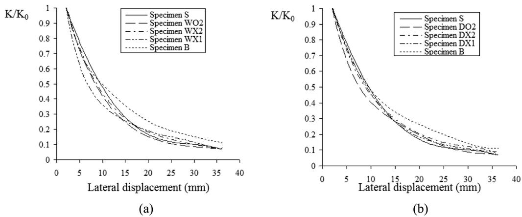
Fig. 11 Reduced stiffness of the infilled frames; (a) Window openings of various locations, (b) Door openings of various locations
