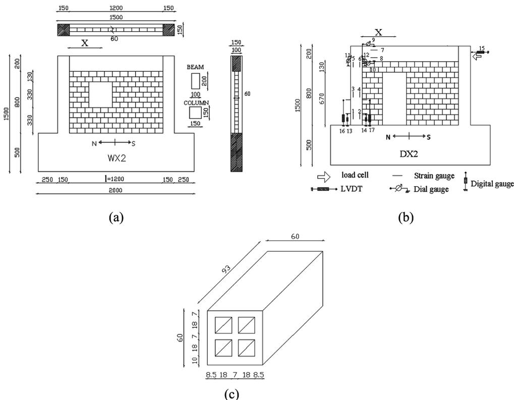
Fig. 2 Description of infilled frame specimens and instrumentation; (a) window opening (mm), (b) door opening (mm), (c) brick unit (mm)
