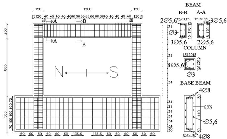
Fig. 1 Reinforcement detailing of the R/C frame model (mm)
