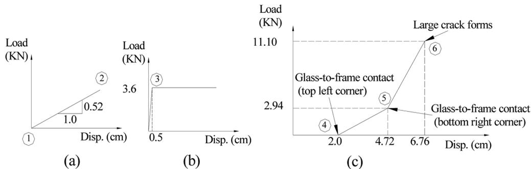
Fig. 8 Simplified load-displacement relations: (a) unglazed frame, (b) uniform gasket/blocking-to-glass friction, (c) after first glass-to-frame contact
