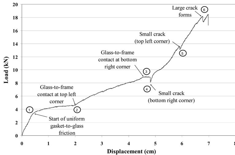
Fig. 4 Load-displacement relationship during static (0.01 cm/sec) racking test
