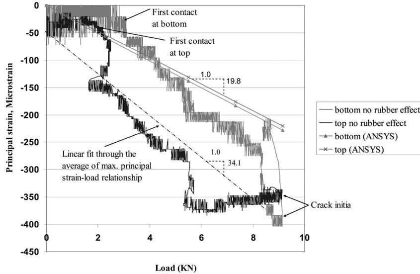
Fig. 9 Maximum principal strain versus contact load
