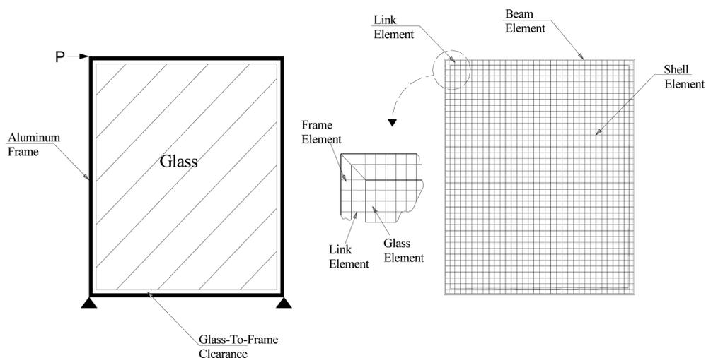
Fig. 5 Schematic diagram of applied load and mesh used for finite element model analysis
