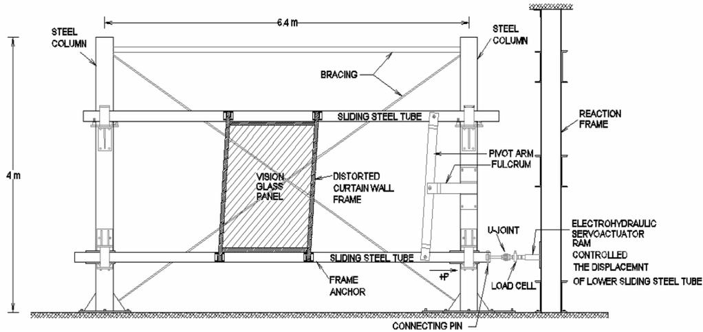
Fig. 2 Dynamic Racking Test Facility schematic
