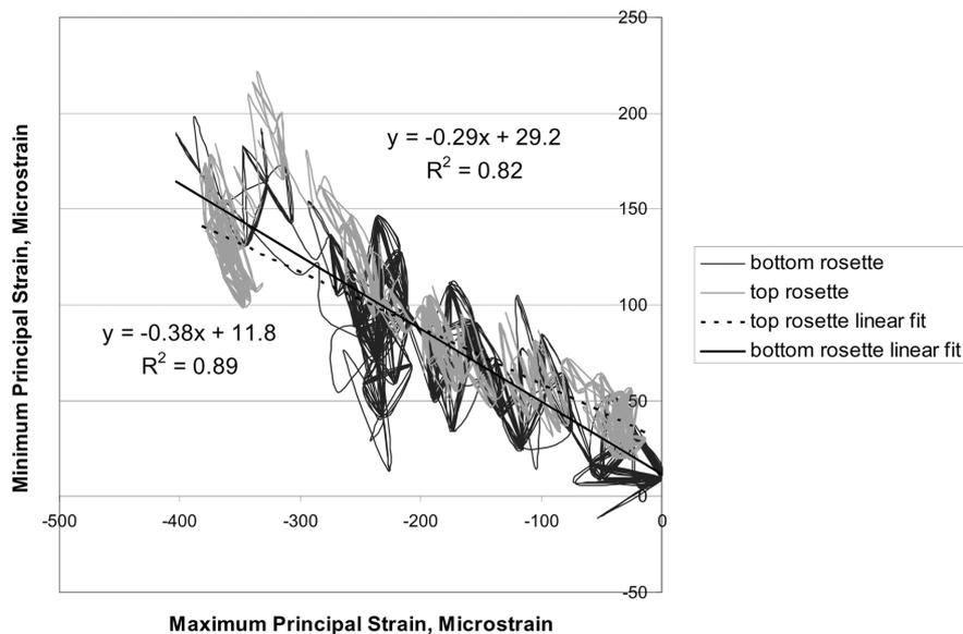
Fig. 11 Relation between principal strains at rosette strain gage locations
