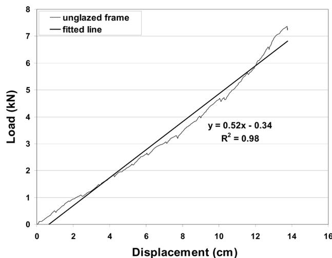
Fig. 7 Load-displacement relationship during static (0.01 cm/sec) racking of unglazed curtain wall frame
