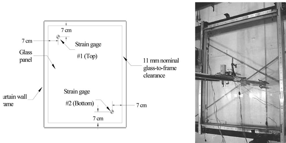
Fig. 3 Strain gage locations on architectural glass curtain wall mock-up
