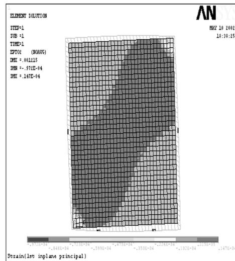
Fig. 10 (a) Comparison of the test and the ANSYS finite element analysis results (Note: Lines for reported strains are scaled relative to each other. Angles are measured from the principal strain direction to the horizon line), (b) Distribution of principal strain at cracking load from finite element analysis (Note: Color contours shows the distribution of the first principal strain)
