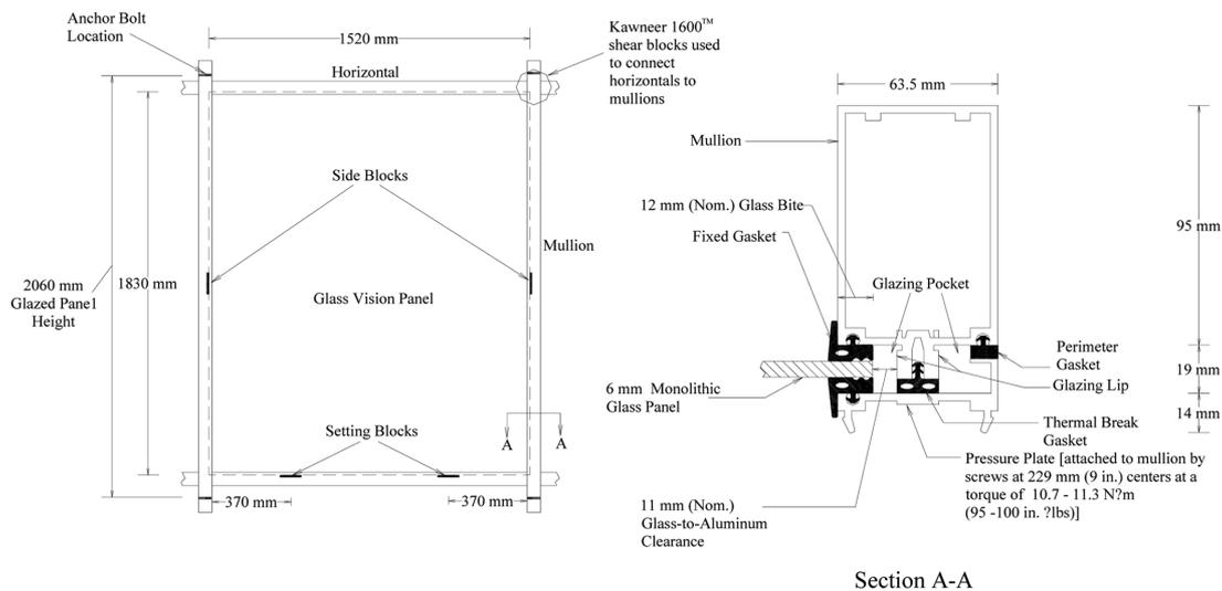
Fig. 1 General glazing details for curtain wall mock-up tested
