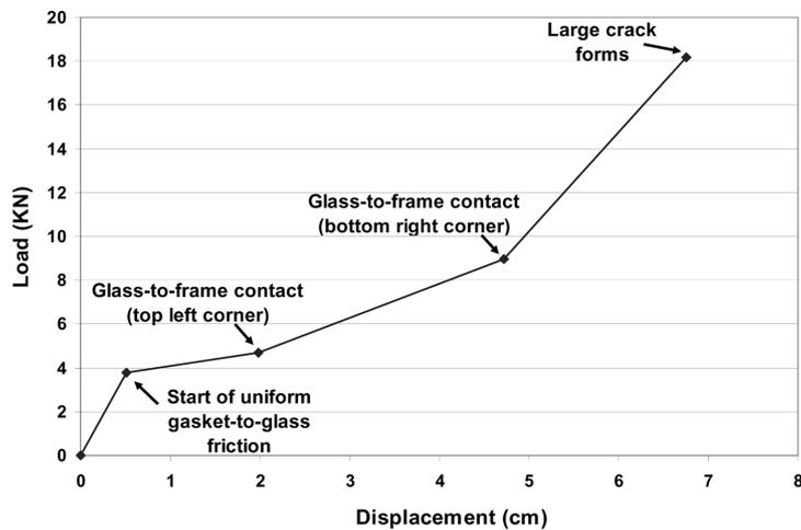
Fig. 6 Simplified load-displacement relationship during static (0.01 cm/sec) racking test
