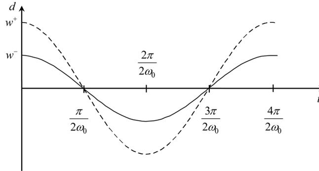
Fig. 3 Free vibration with fuzzy initial displacement
