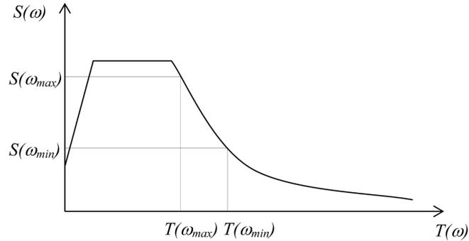
Fig. 2 Example of pseudoacceleration spectrum
