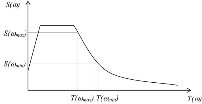
Fig. 2 Example of pseudoacceleration spectrum
