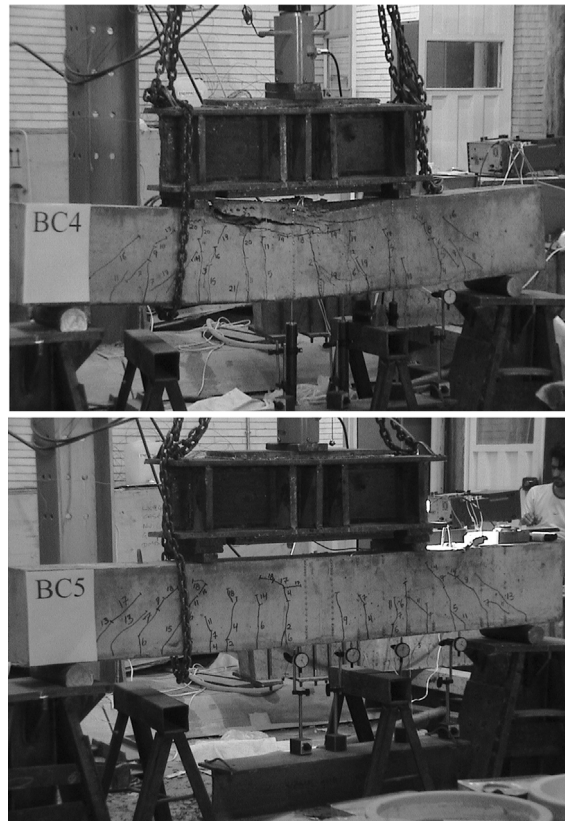
Fig. 2 Crack propagation and failure of the beams under load
