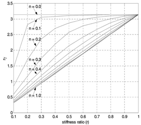
Fig. 3(b) Dimensionless buckling load over a region  $(0 < r \leq 1, 0 \leq n \leq 1)$  for different values of length ratio
