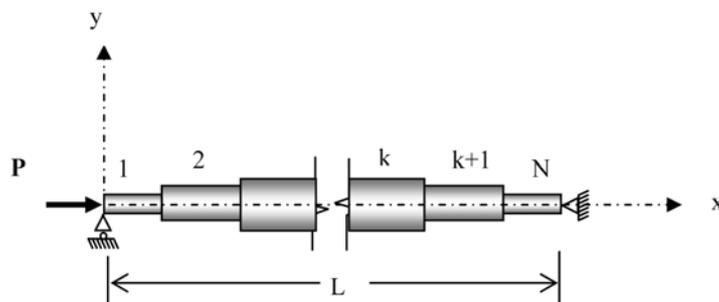
Fig. 1 A general layout of a multi-segments compression member
