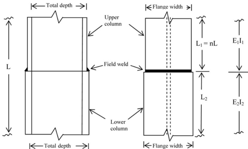
Fig. 5 Directly welded column splice
