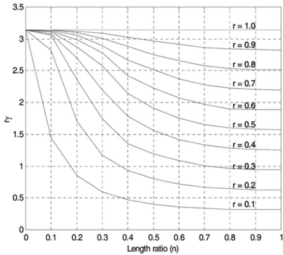
Fig. 3(a) Dimensionless buckling load over a region  $(0 < r \leq 1, 0 \leq n \leq 1)$  for different values of stiffness ratio
