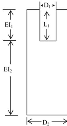
Fig. 8 Compression member with a service duct
