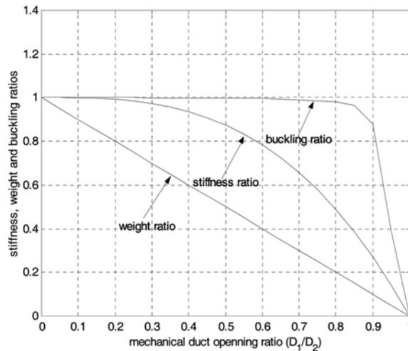
Fig. 9 Stiffness, weight and buckling load ratios of a column with service duct ( $n = 0.1$ )
