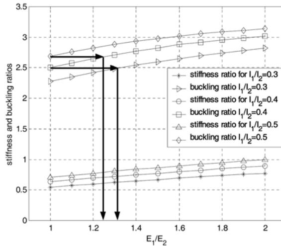
Fig. 10 Stiffness and buckling load ratios of a column with section and material variability ( $n = 0.4$ )
