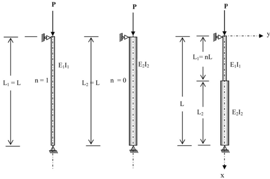
Fig. 2 Two-steps compression member with piecewise constant cross section ( $0 \leq n \leq 1$ )
