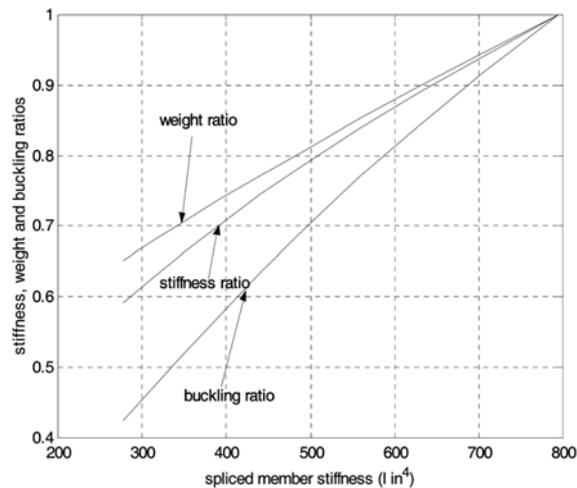
Fig. 7 Stiffness, weight and buckling load ratios of spliced W-shaped column ( $n = 0.6$ )
