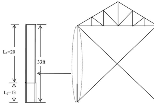
Fig. 6 A spliced column as part of an industrial building
