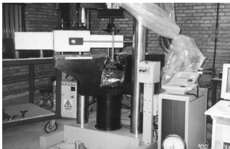
Fig. 14 Column specimen under testing by 1000 kN Dartec Universal Testing Machine
