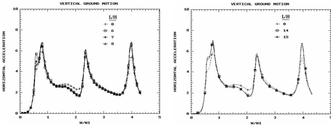
Fig. 4 Horizontal accelerations at dam crest due to vertical ground motion for two sets of moderate and high values of normalized rigorous fluid-foundation interaction length
