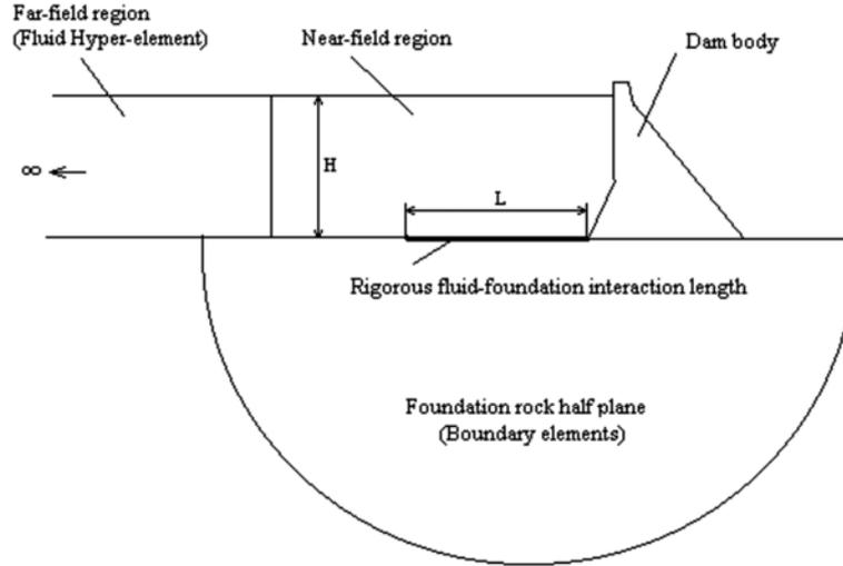
Fig. 1 Dam-reservoir-foundation system (Schematic representation)
