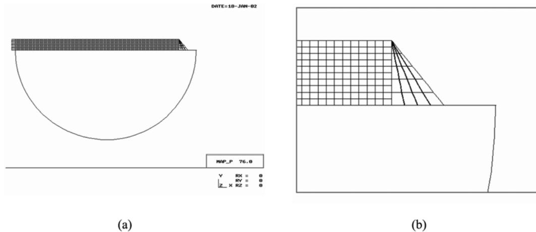
Fig. 2 Dam-reservoir-foundation system: (a) Complete model, (b) Close-up view
