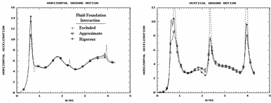
Fig. 5 Horizontal accelerations at dam crest due to horizontal and vertical ground motions ( $E_f/E_d = 2$ )
