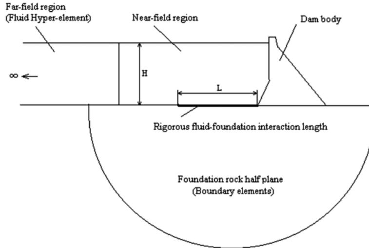
Fig. 1 Dam-reservoir-foundation system (Schematic representation)
