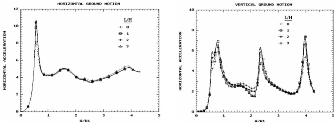
Fig. 3 Horizontal accelerations at dam crest due to horizontal and vertical ground motions for low values of normalized rigorous fluid-foundation interaction length
