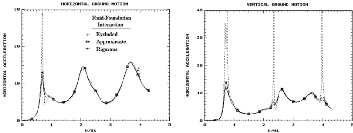
Fig. 8 Horizontal accelerations at dam crest due to horizontal and vertical ground motions (Fictitious cases:  $E_f/E_d = 1$  and rigid dam base)
