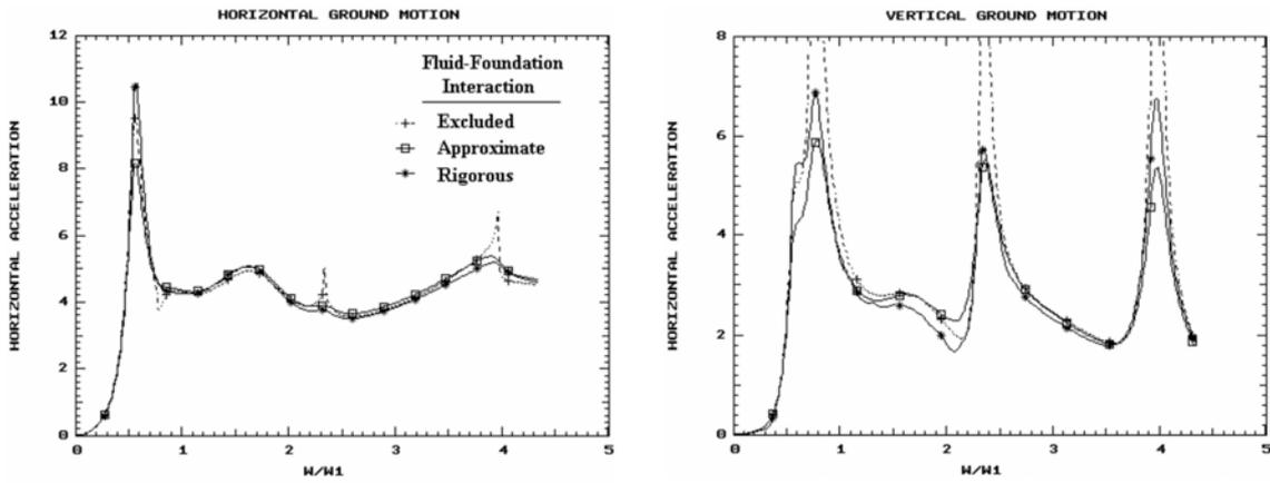
Fig. 6 Horizontal accelerations at dam crest due to horizontal and vertical ground motions ( $E_f/E_d = 1$ )
