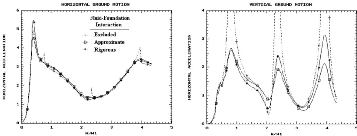
Fig. 7 Horizontal accelerations at dam crest due to horizontal and vertical ground motions ( $E_f/E_d = 1/4$ )
